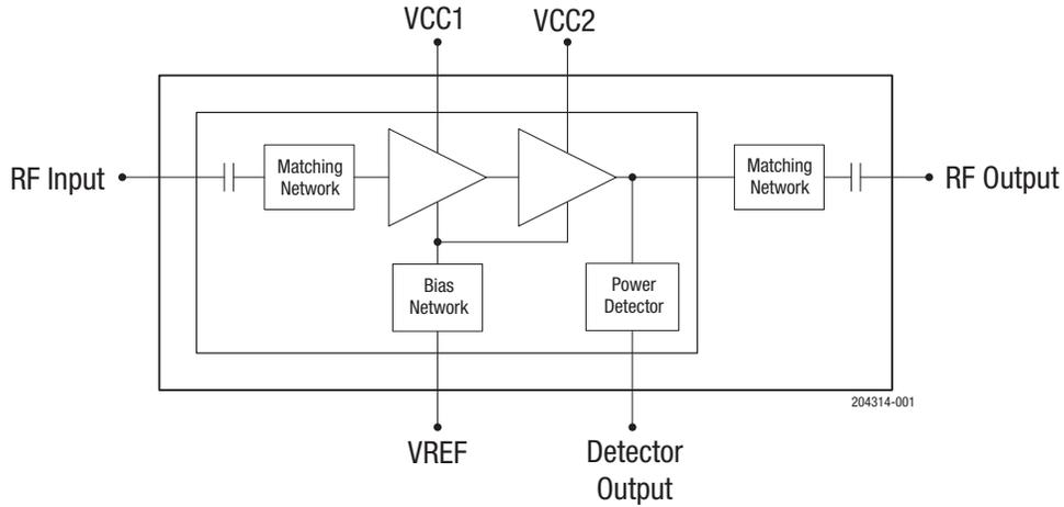
Figure 1. AWB7124 Block Diagram
