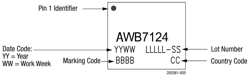
Figure 5. AWB7124 Typical Part Markings (Top View)
