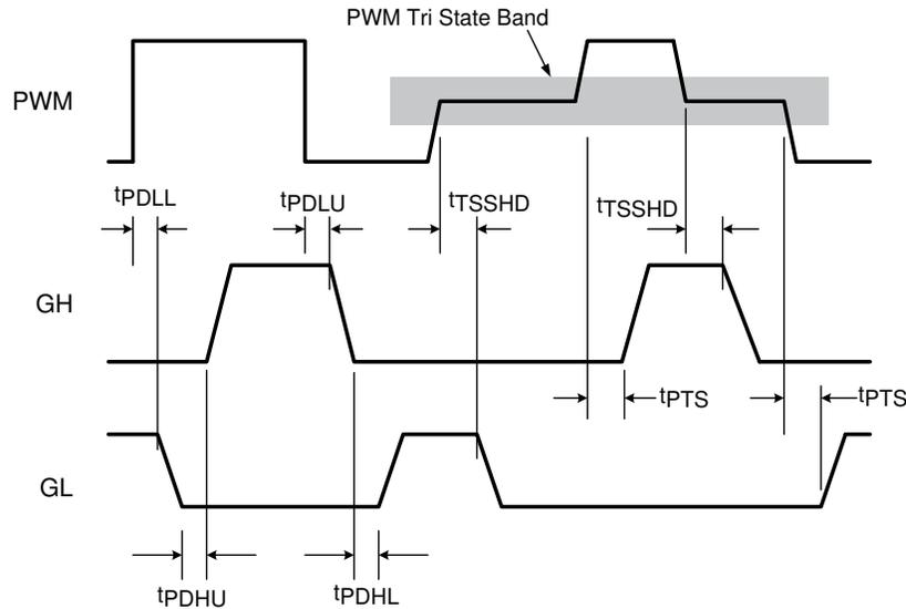
Figure 13. Timing Diagram
