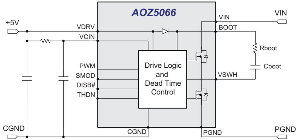
Figure 14. Applying VDRV and Generating BOOT Supply
