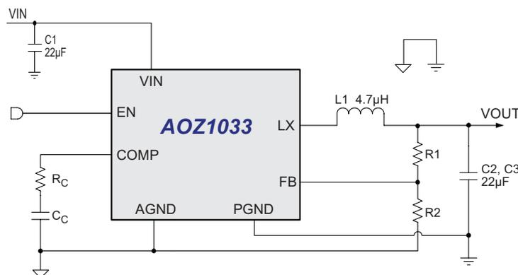
Figure 1. 3.3V 3A Synchronous Buck Regulator
