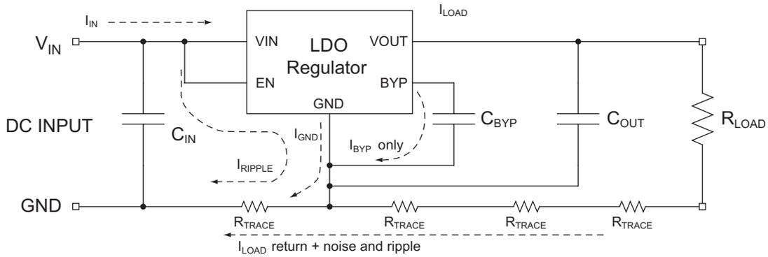
Figure 2: Recommended LDO Regulator Layout.
