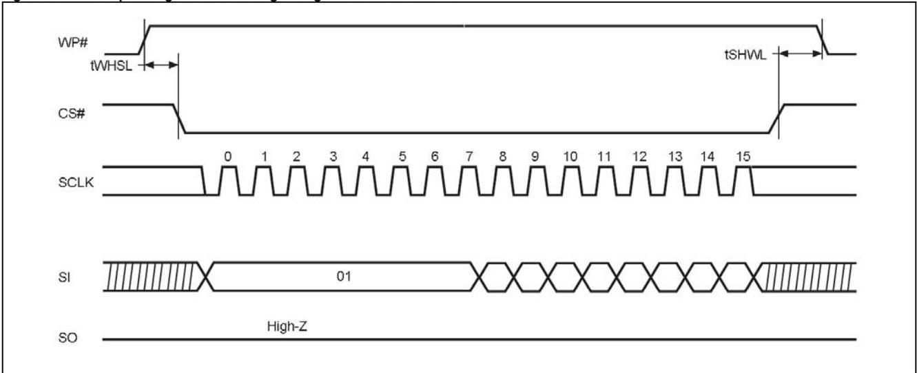
Figure 9. Write Enable (WREN) Sequence (Command 06)
