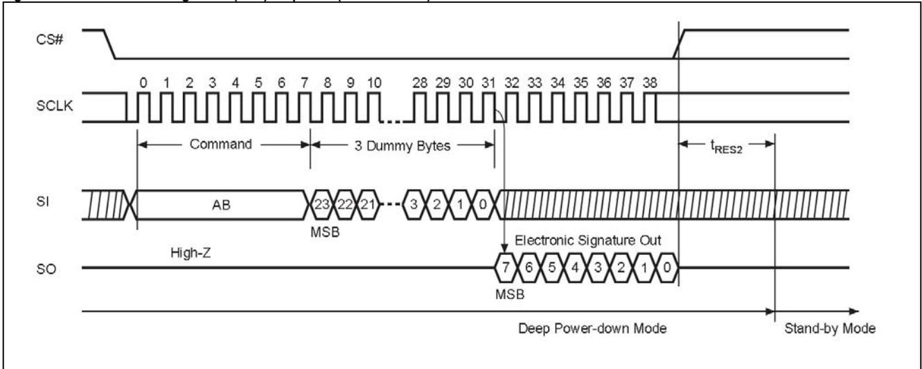
**Figure 26. Release from Deep Power-down (RDP) Sequence (Command AB)**
