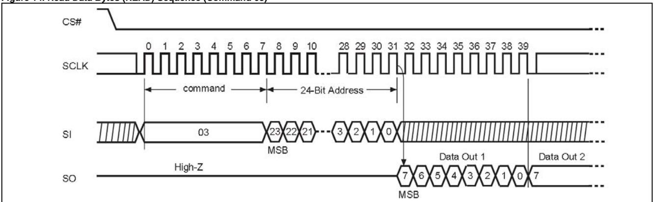
**Figure 15. Read at Higher Speed (FAST\_READ) Sequence (Command 0B)**
