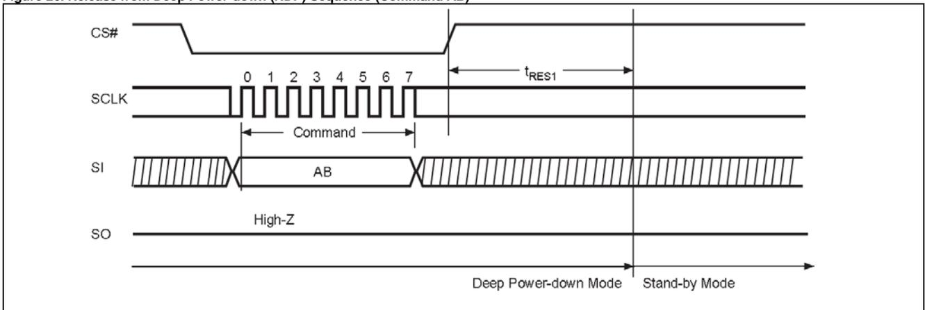
**Figure 27. Read Electronic Manufacturer & Device ID (REMS) Sequence (Command 90 or EF or DF)**
