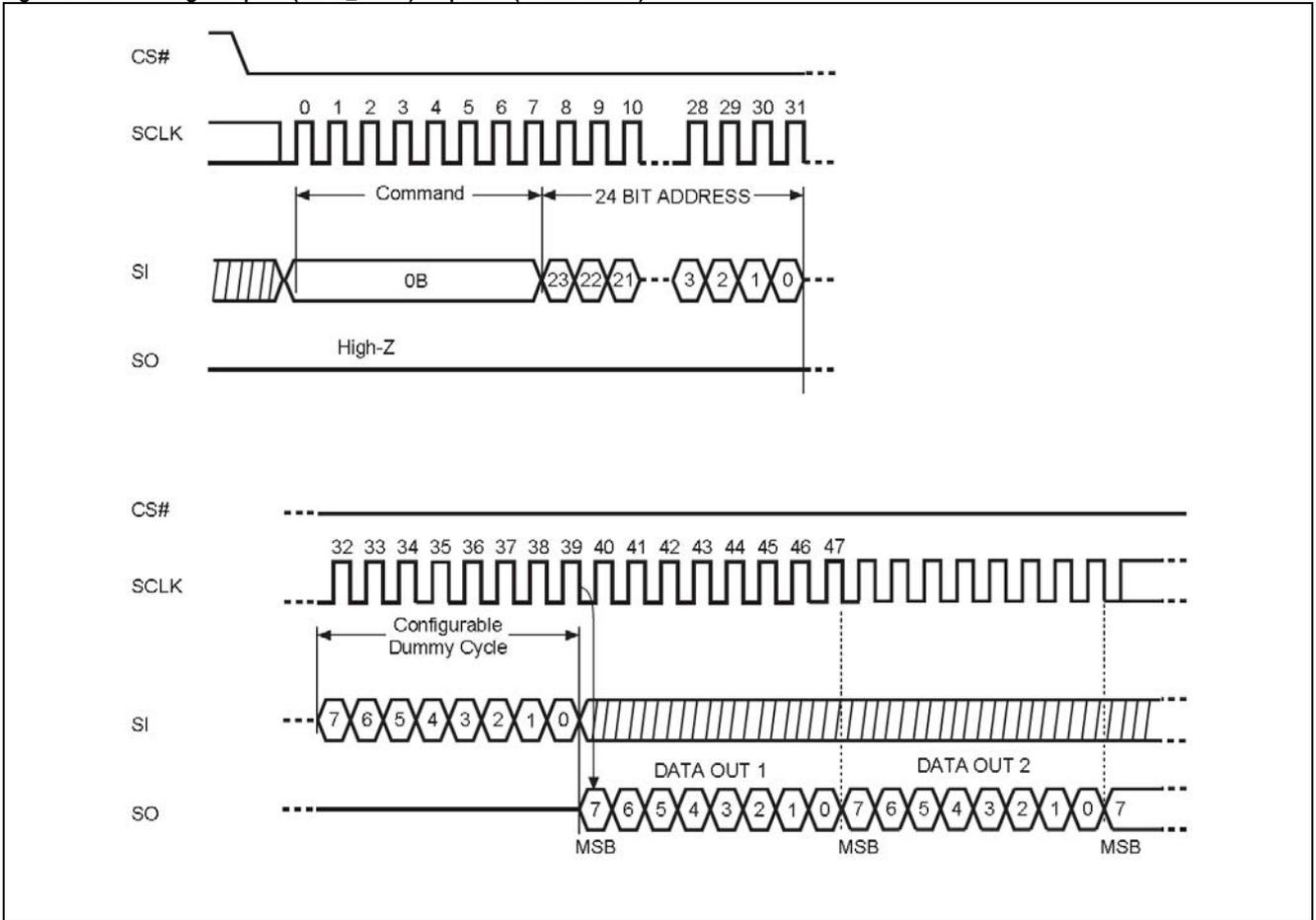
**Figure 16. 2 x I/O Read Mode Sequence (Command BB)**
