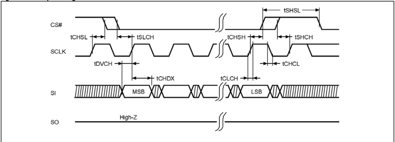
Figure 7. Output Timing
