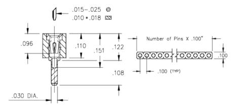
**Description:** Interconnect Socket Low Profile Solder Tail Socket Accepts .015" - .025" (0,38 - 0,635 mm) dia leads Single Row Through Hole Plating Code: Shell Plating:
