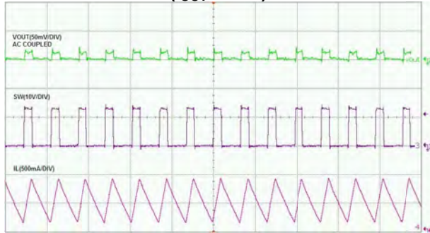
Steady State Test ( I_{OUT} = 0.5A )
