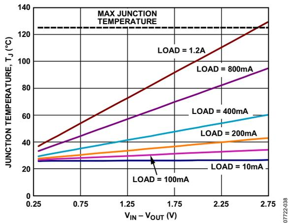
Figure 42. 500 mm<sup>2</sup> of PCB Copper,  $T_B = 25^\circ\text{C}$ , LFCSP
