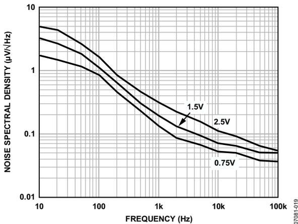
Figure 19. Noise Spectral Density vs. Output Voltage, I<sub>LOAD</sub> = 10 mA
