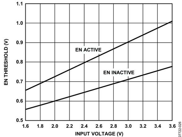
Figure 29. Typical  $EN$  Pin Thresholds vs. Input Voltage
