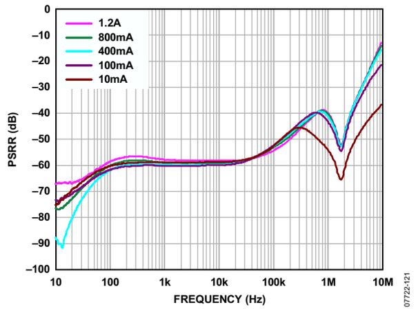
Figure 21. Power Supply Rejection Ratio vs. Frequency, V<sub>OUT</sub> = 1.5 V, V<sub>IN</sub> = 2.5 V
