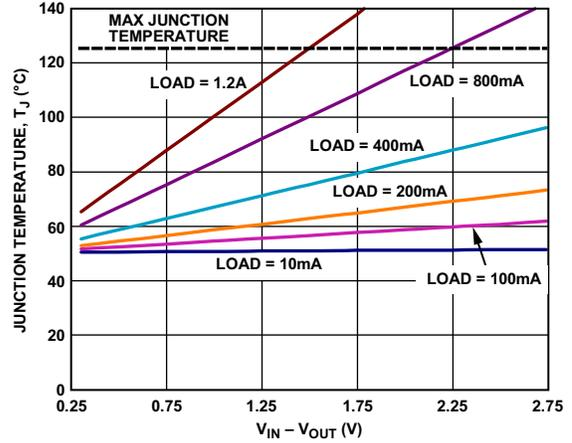
Figure 39. 6400 mm<sup>2</sup> of PCB Copper, T<sub>A</sub> = 50°C, LFCSP
