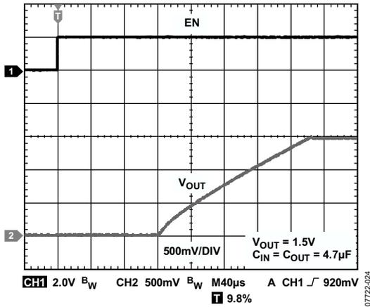
Figure 27.  $V_{OUT}$  Ramp-Up with Internal Soft Start
