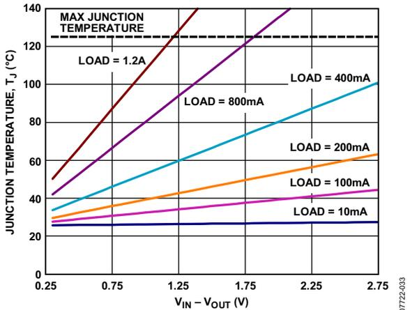
Figure 37. 500 mm<sup>2</sup> of PCB Copper, T<sub>A</sub> = 25°C, LFCSP
