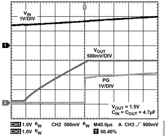
Figure 30. Typical PG Behavior vs. V<sub>OUT</sub>, V<sub>IN</sub> Rising (V<sub>OUT</sub> = 1.5 V)
