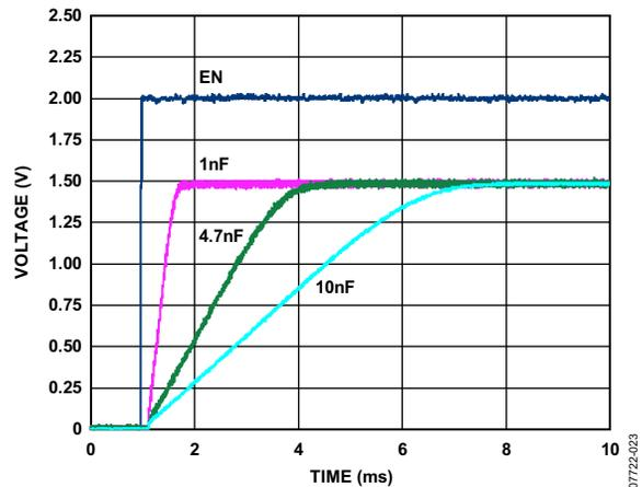
Figure 26.  $V_{OUT}$  Ramp-Up with External Soft Start Capacitor
