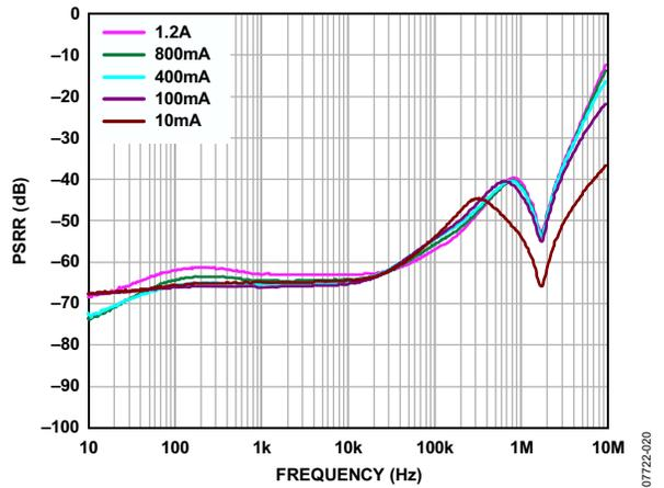
Figure 20. Power Supply Rejection Ratio vs. Frequency, V<sub>OUT</sub> = 0.75 V, V<sub>IN</sub> = 1.75 V
