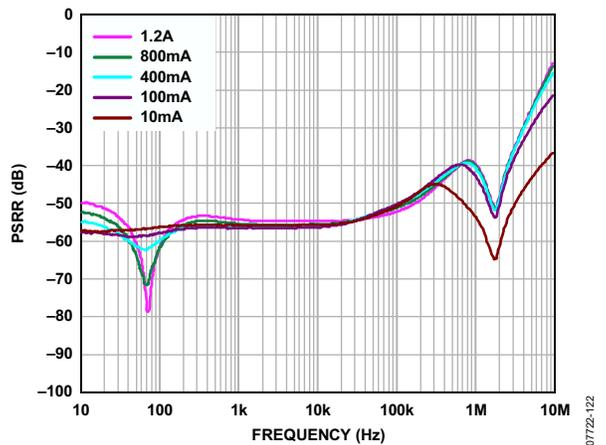
Figure 22. Power Supply Rejection Ratio vs. Frequency, V<sub>OUT</sub> = 2.5 V, V<sub>IN</sub> = 3.5 V
