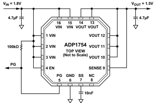
Figure 1. ADP1754 with Fixed Output Voltage, 1.5 V
