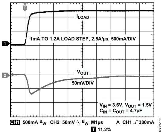
Figure 33. Output Transient Response,  $C_{OUT} = 4.7 \mu\text{F}$
