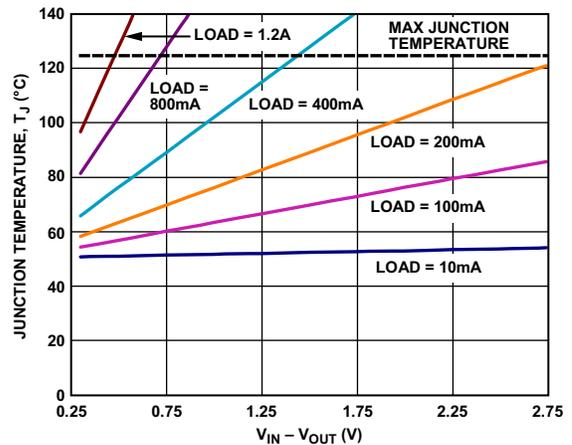
Figure 41. 0 mm<sup>2</sup> of PCB Copper, T<sub>A</sub> = 50°C, LFCSP
