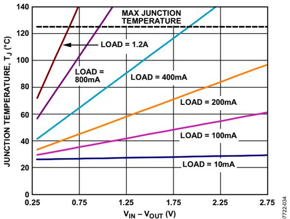
Figure 38. 0 mm<sup>2</sup> of PCB Copper, T<sub>A</sub> = 25°C, LFCSP
