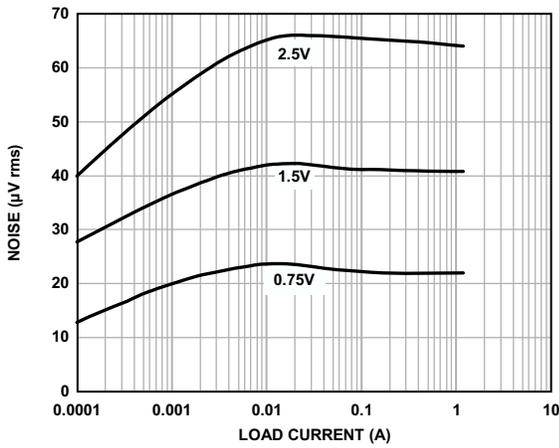
Figure 18. Noise vs. Load Current and Output Voltage
