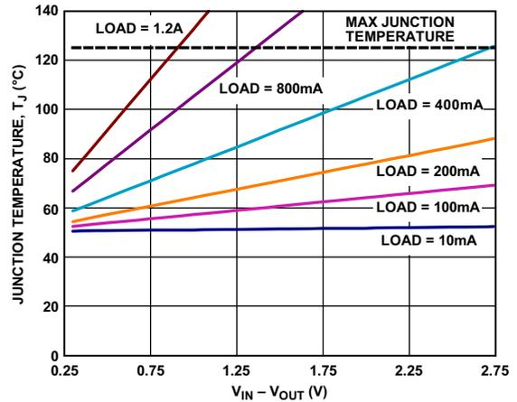
Figure 40. 500 mm<sup>2</sup> of PCB Copper, T<sub>A</sub> = 50°C, LFCSP
