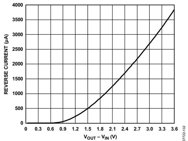
Figure 32. Reverse Current vs. V<sub>OUT</sub> - V<sub>IN</sub>
