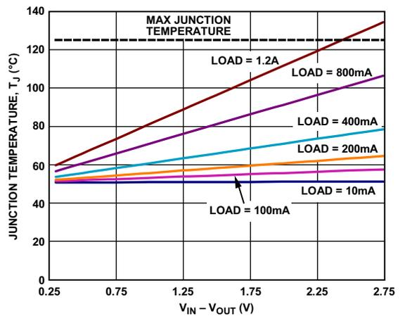
Figure 45. 1000 mm<sup>2</sup> of PCB Copper,  $T_B = 50^\circ\text{C}$ , LFCSP
