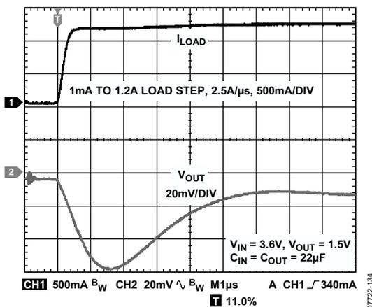
Figure 34. Output Transient Response,  $C_{OUT} = 22 \mu\text{F}$
