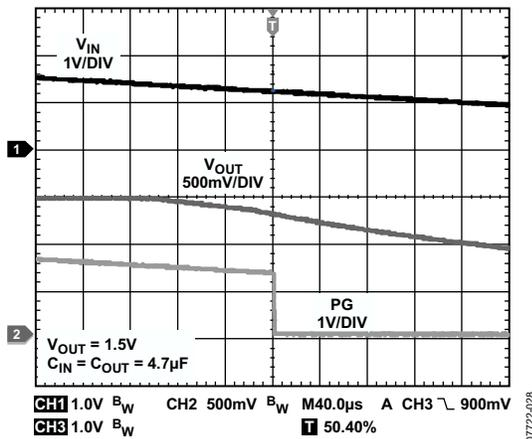
Figure 31. Typical PG Behavior vs. V<sub>OUT</sub>, V<sub>IN</sub> Falling (V<sub>OUT</sub> = 1.5 V)
