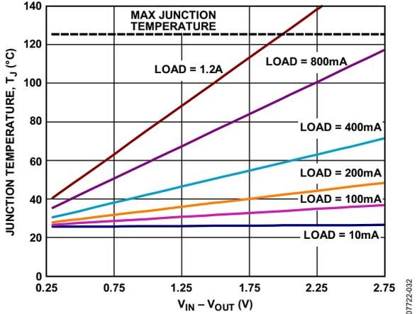
Figure 36. 6400 mm<sup>2</sup> of PCB Copper, T<sub>A</sub> = 25°C, LFCSP
