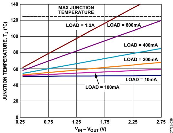
Figure 43. 500 mm<sup>2</sup> of PCB Copper,  $T_B = 50^\circ\text{C}$ , LFCSP
