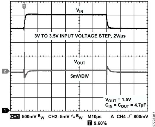
Figure 17. Line Transient Response, Load Current = 1200 mA
