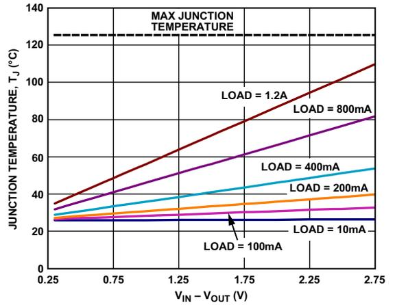
Figure 44. 1000 mm<sup>2</sup> of PCB Copper,  $T_B = 25^\circ\text{C}$ , LFCSP
