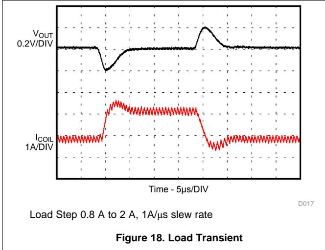
Figure 18. Load Transient
