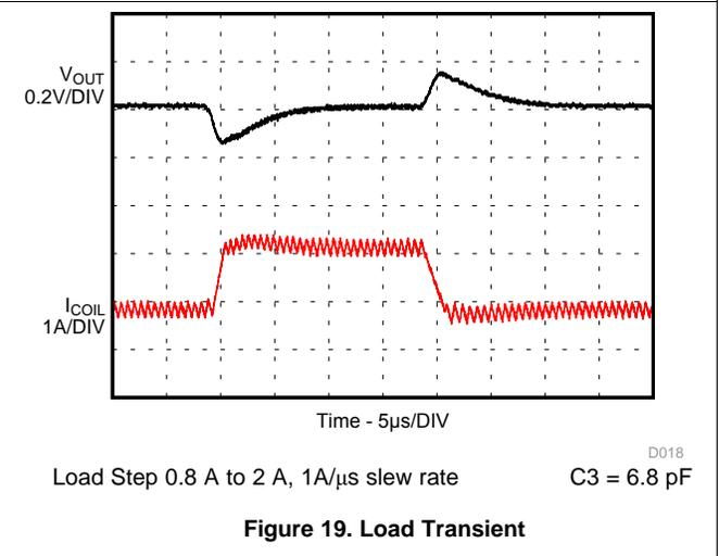
Figure 19. Load Transient
