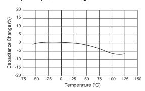
[ Example of Temperature Characteristics X5R(R6) ] Sample: 22µF, Rated Voltage 4VDC
