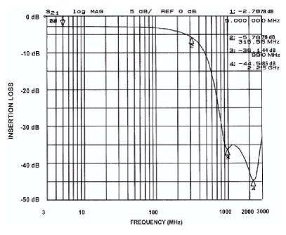
Figure 2. Insertion Loss vs. Frequency (Pins 2 and 15)
