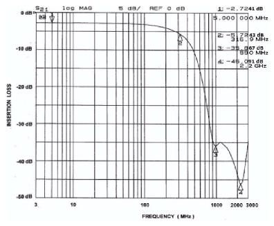
Figure 1. Insertion Loss vs. Frequency (Pins 1 and 16)
