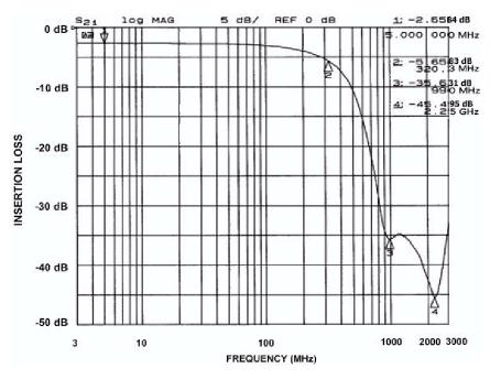
Figure 3. Insertion Loss vs. Frequency (Pins 3 and 14)
