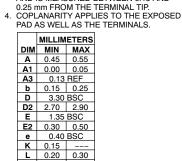
DIMENSIONING AND TOLERANCING PER ASME Y14.5M, 1994. CONTROLLING DIMENSION: MILLIMETERS.
