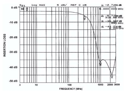
Figure 5. Insertion Loss vs. Frequency (Pins 7 and 10)
