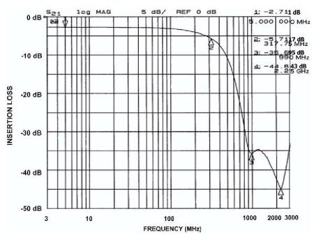
Figure 4. Insertion Loss vs. Frequency (Pins 6 and 11)
