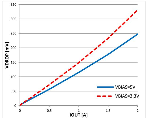
$V_{DROPP}$  vs.  $V_{BIAS}$  @  $V_{OUT}=1.2V$
