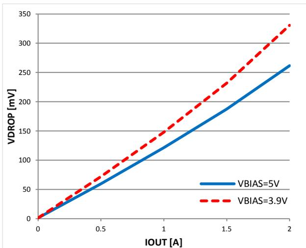
$V_{DROPP}$  vs.  $V_{BIAS}$  @  $V_{OUT}=1.8V$
