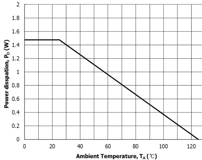
The graph above is valid for the thermal impedance specified in the Absolute Maximum Ratings section on page 1.
