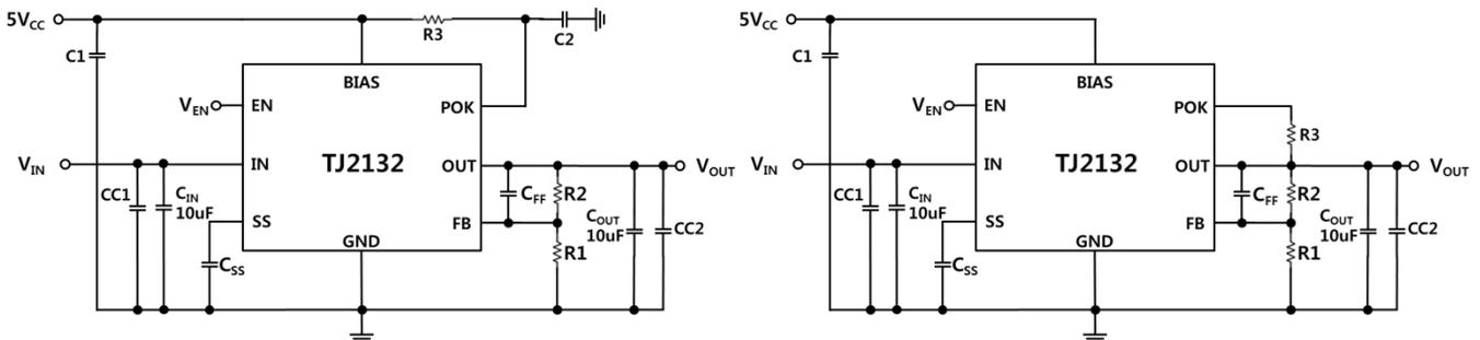
Fig.1 Application with Decoupling & Feed-Forward Capacitor
