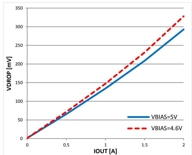
$V_{DROPP}$  vs.  $V_{BIAS}$  @  $V_{OUT}=2.5V$
