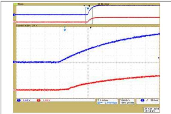
**FIGURE 2-36:** 50 k $\Omega$  – Power-Up Wiper Response Time (1  $\mu\text{s}/\text{Div}$ ).
