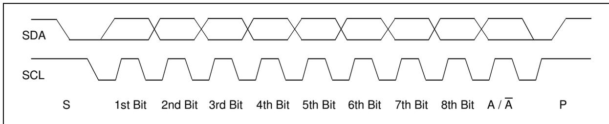
**FIGURE 6-7:** Typical 8-Bit I<sup>2</sup>C Waveform Format.
