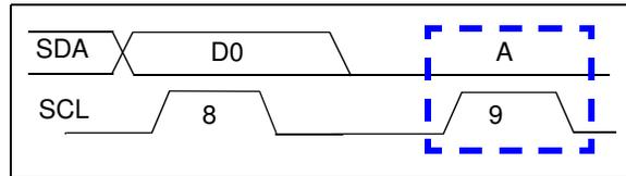
**FIGURE 6-4:** Acknowledge Waveform.
