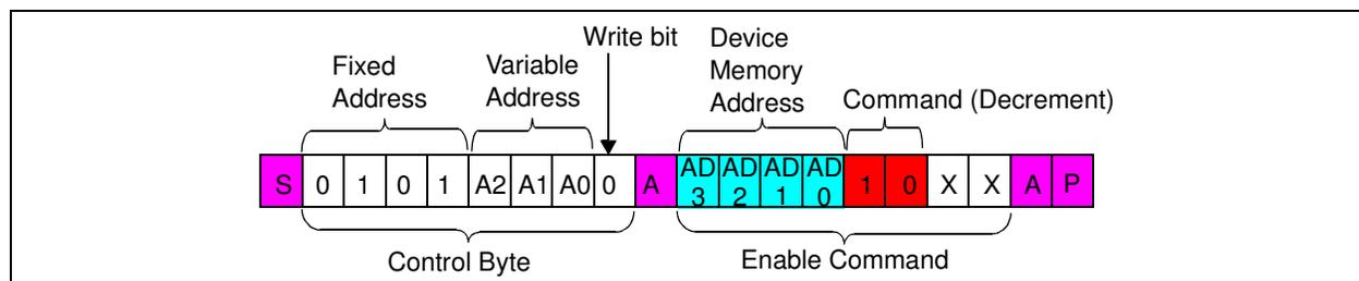
**FIGURE 7-10:** I<sup>2</sup>C Enable Command Sequence.
