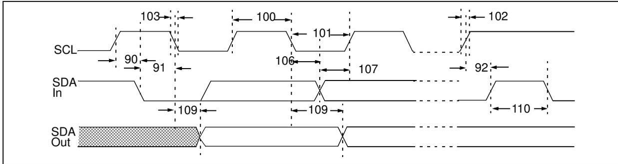
**FIGURE 1-2:** I<sup>2</sup>C Bus Data Timing.
