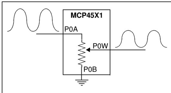
**FIGURE 8-5:** Signal Attenuation Block Diagram - Ground Referenced.
