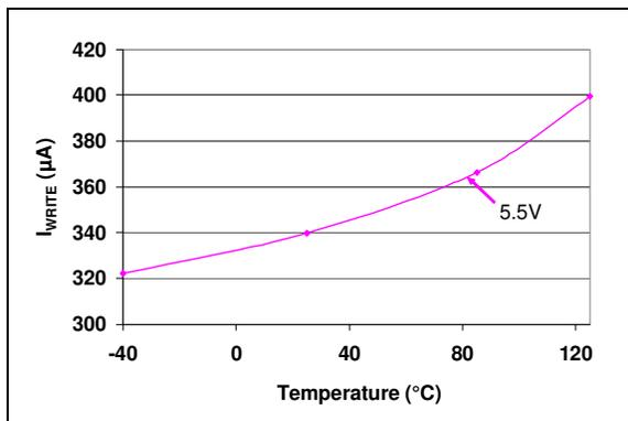
**FIGURE 2-3:** Write Current ( $I_{WRITE}$ ) vs. Ambient Temperature.
