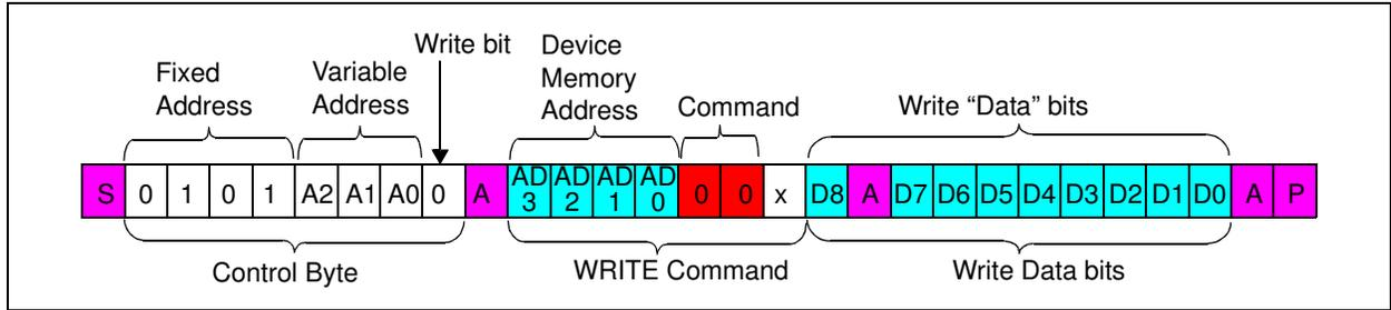
**FIGURE 7-2:** I<sup>2</sup>C Write Sequence.
