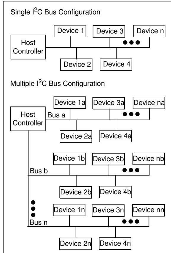
**FIGURE 8-3:** Typical Application I<sup>2</sup>C Bus Configurations.
