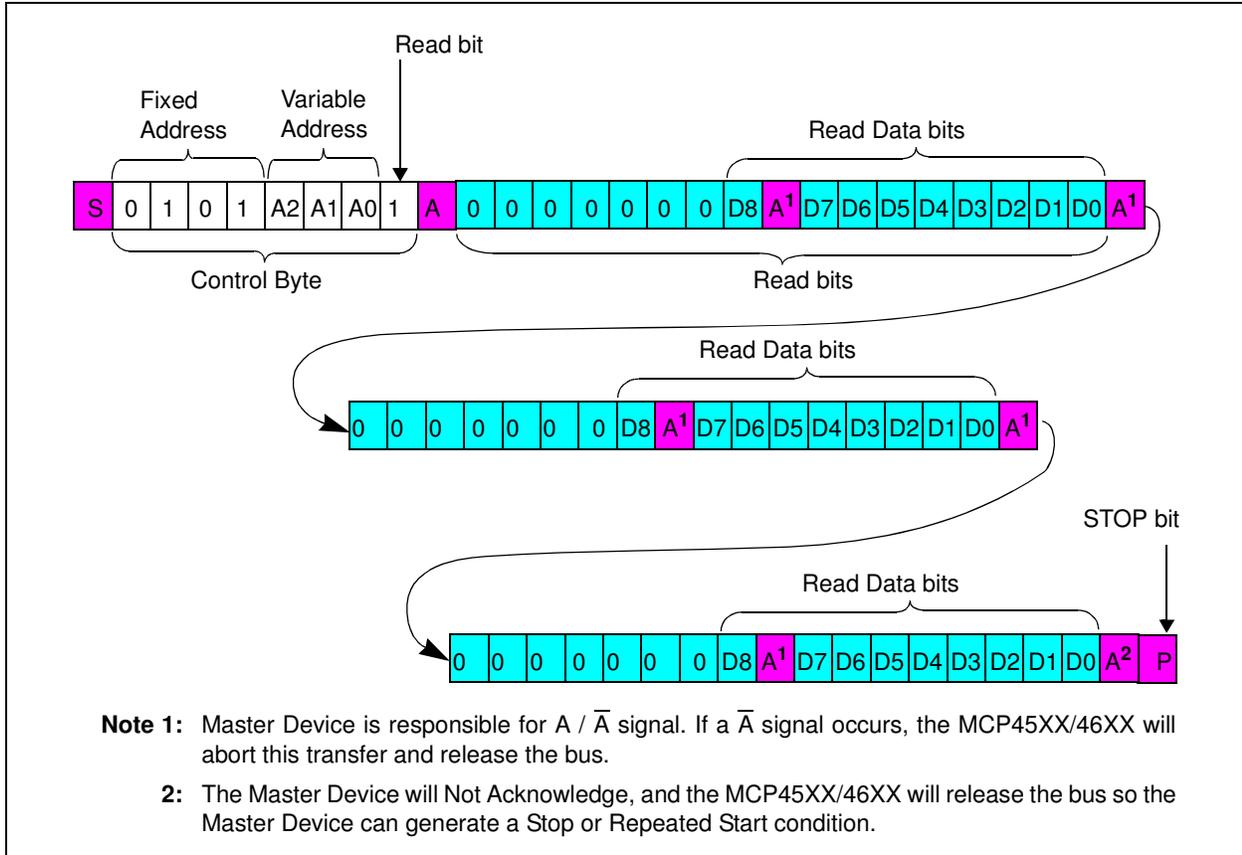
**FIGURE 7-6:** I<sup>2</sup>C Continuous Reads.
