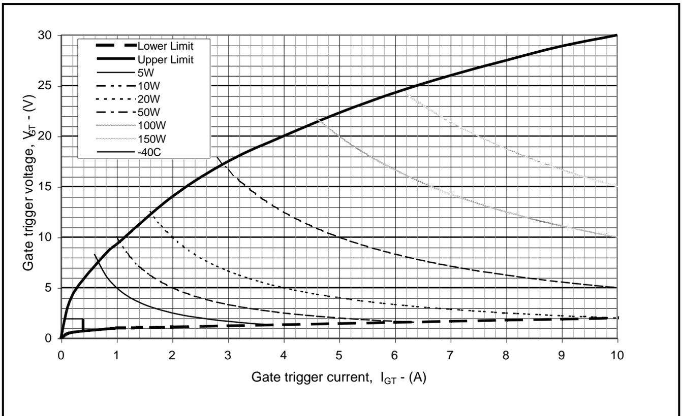
Fig. 15 Gate characteristics
