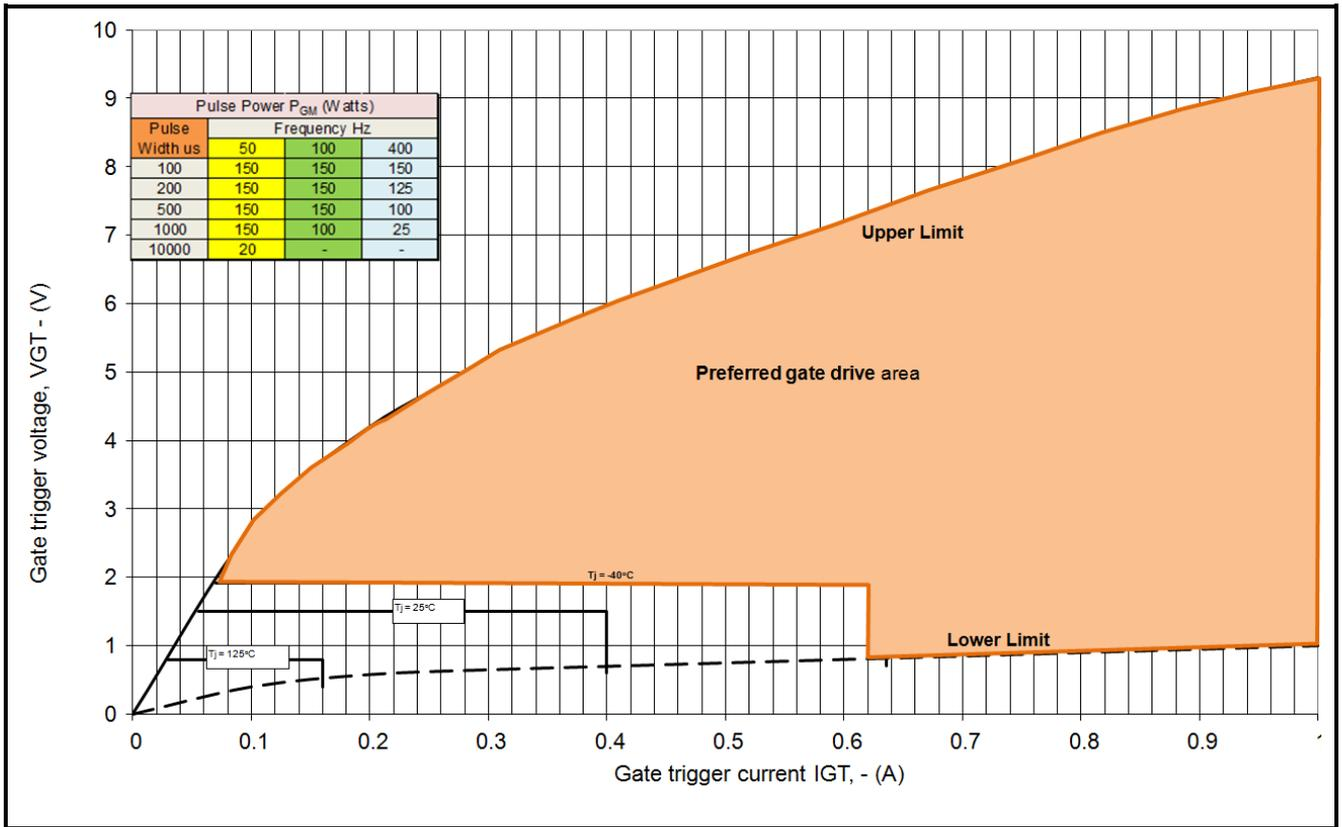
Fig14 Gate Characteristics
