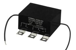
Style SCC is ideal for use in medium to high current applications where a dual IGBT module is used. This low loss snubber directly reduces turn-off voltage overshoots and is effective in reducing turn-on voltage transients.
