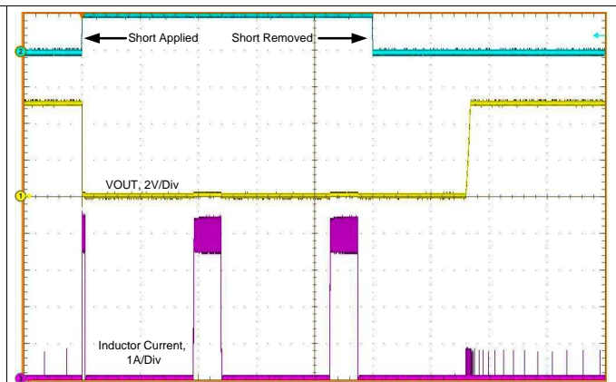
Figure 12. Short-Circuit Transient and Recovery
