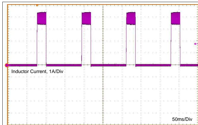
Figure 11. Inductor Current Burst in Short-Circuit Mode
