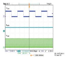
Fig.12 1kHz PWM Dimming Waveform
