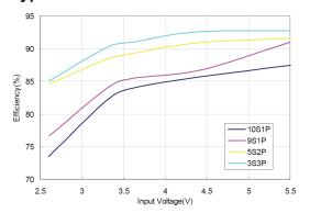
Fig.1 Efficiency VS Input Voltage (L=10µH)
