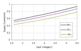
Fig.6 Supply Current VS Input Voltage
