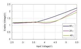
Fig.8 Enable Voltage VS Input Voltage
