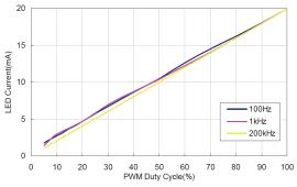
Fig.3 LED Current VS PWM Dimming(10S1P LEDs)
