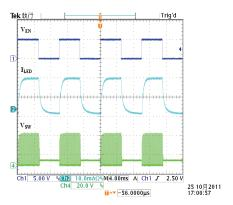
Fig.11 200Hz PWM Dimming Waveform
