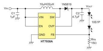
Fig.13 Application for Driving 10S1P WLEDs
