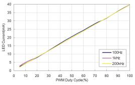
Fig.4 LED Current VS PWM Di
