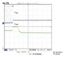
Fig.10 Open LED Protection
