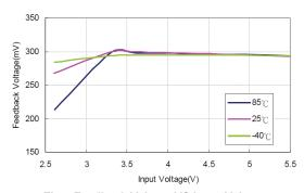
Fig.7 Feedback Voltage VS Input Voltage
