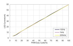
Fig.5 LED Current VS PWM Dimming (3S3P LEDs)
