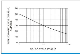
Fig.2- MAXIMUM NON-REPETITIVE PEAK FORWARD SURGE CURRENT
