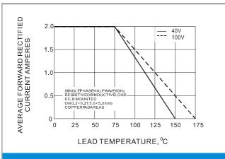
Fig.1-FORWARD CURRENT DERATING CURVE
