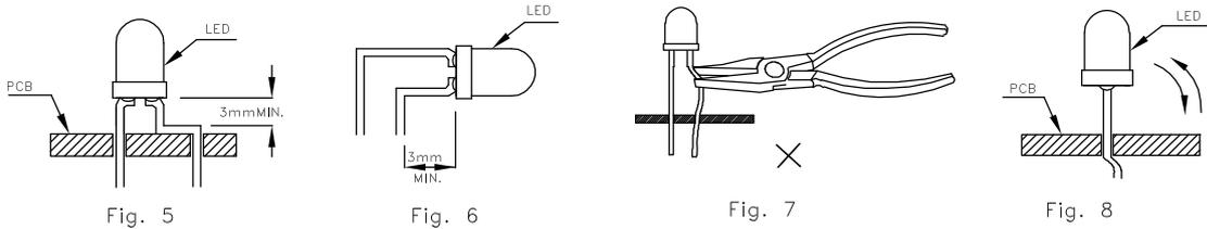
8. During soldering, component covers and holders should leave clearance to avoid placing damaging stress on the LED during soldering.
