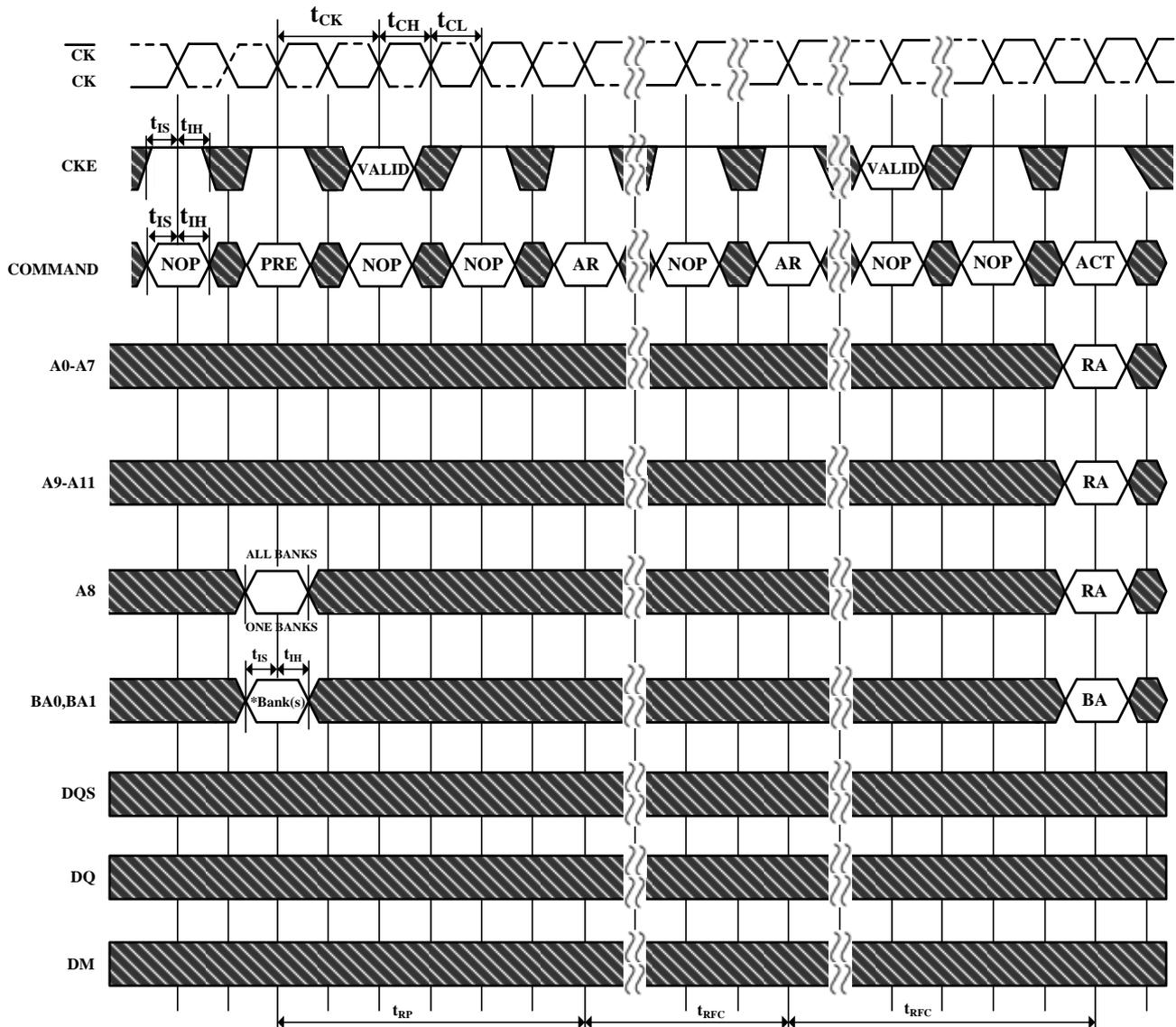
\* = Don't Care, if A8 is HIGH at this point; A8 must be HIGH if more than one bank is active (i.e., must precharge all active banks)
