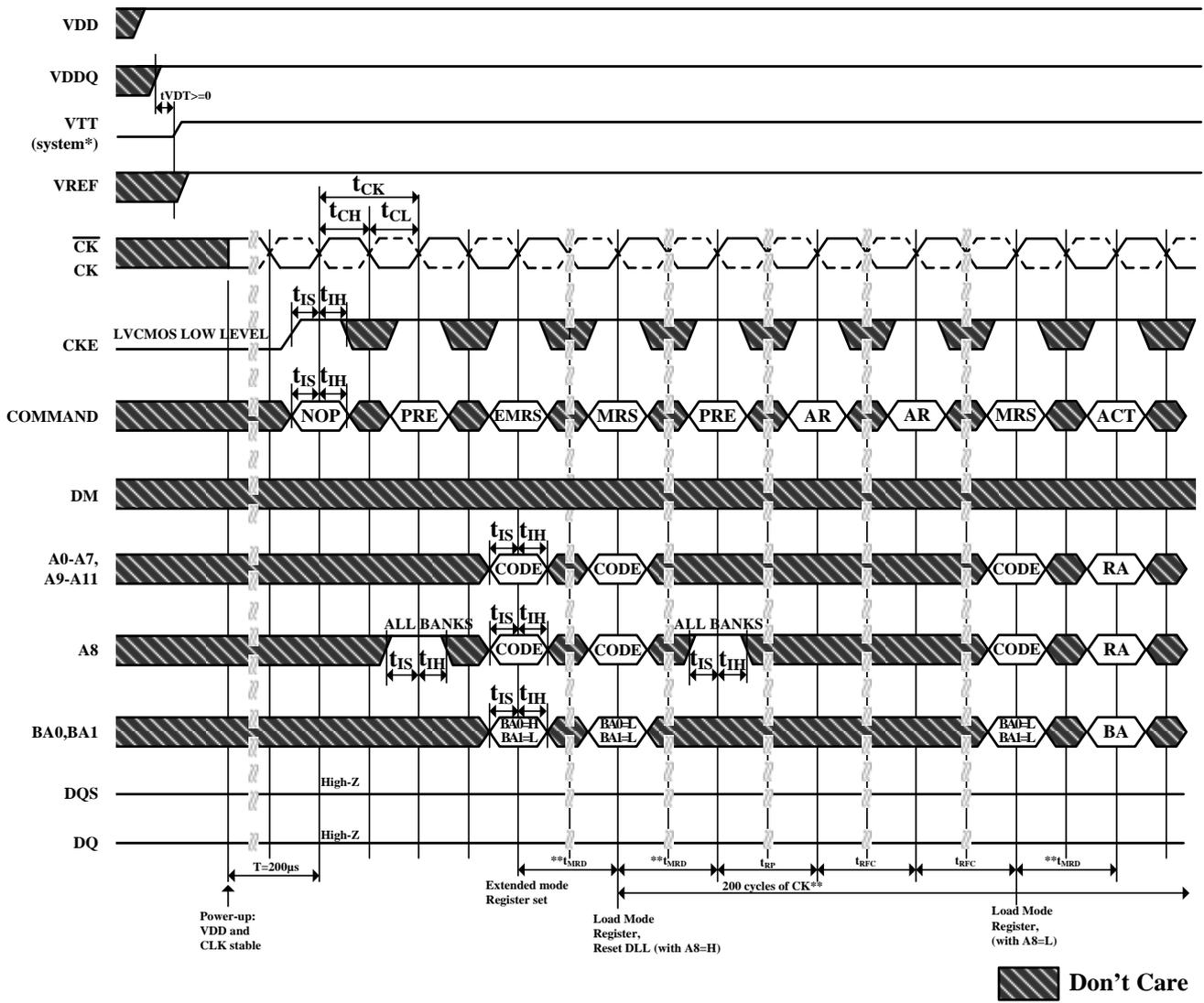
\*=VTT is not applied directly to the device, however  $t_{VID}$  must be greater than or equal to zero to avoid device latch-up.
