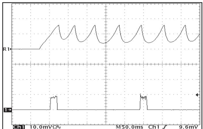
Figure 18: Load Current ( $50A/div$ ) as a function of time when the converter attempts to turn on into a  $1m\Omega$  short circuit. Top trace ( $500\mu s/div$ ) is an expansion of the on-time portion of the bottom trace.  $V_{in} = 48V$
