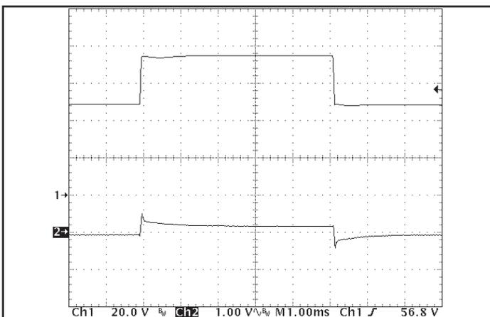
Figure 17: Load Current ( $50A/div$ ) as a function of time when the converter attempts to turn on into a  $1m\Omega$  short circuit. Top trace ( $500\mu s/div$ ) is an expansion of the on-time portion of the bottom trace.  $V_{in} = 48V$
