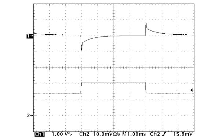
Figure 12: Output voltage response to step-change in load current (50%-75%-50%) of  $I_{out}$  (max);  $di/dt$  = 1A/µs. Load cap 15µF, 100mΩ ESR tantalum capacitor and 1µF ceramic capacitor. Ch 1:  $V_{out}$  (1V/div), Ch 2:  $I_{out}$  (20A/div).  $V_{in}$  = 48V
