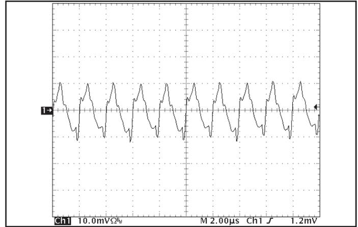
Figure 14: Input Terminal Ripple Current,  $i_c$ , at full rated output current and nominal input voltage with a  $10\mu H$  source impedance and  $47\mu F$  electrolytic capacitor ( $200mA/div$ ). See Figure 13.
