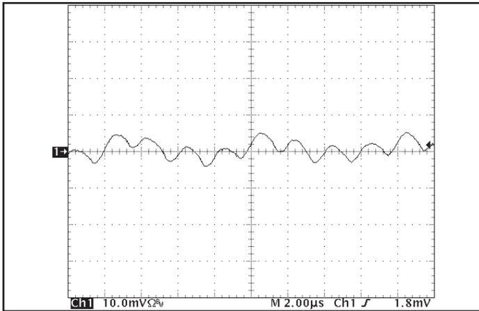
Figure 15: Input reflected ripple current,  $i_s$ , through a  $10\mu H$  source inductor; using a  $47\mu F$  electrolytic input capacitor ( $20mA/div$ ) at nominal input voltage and rated load current. See Figure 13.
