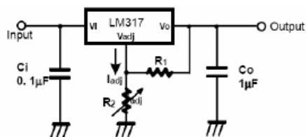
C<sub>i</sub> is required when regulator is located an appreciable distance from power supply filter.
