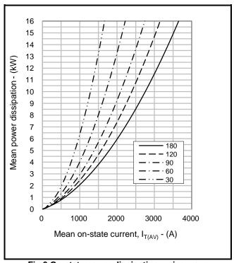
Fig.3 On-state power dissipation – sine wave
