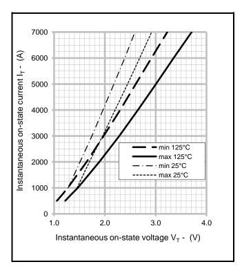
Fig.2 Maximum & minimum on-state characteristics
