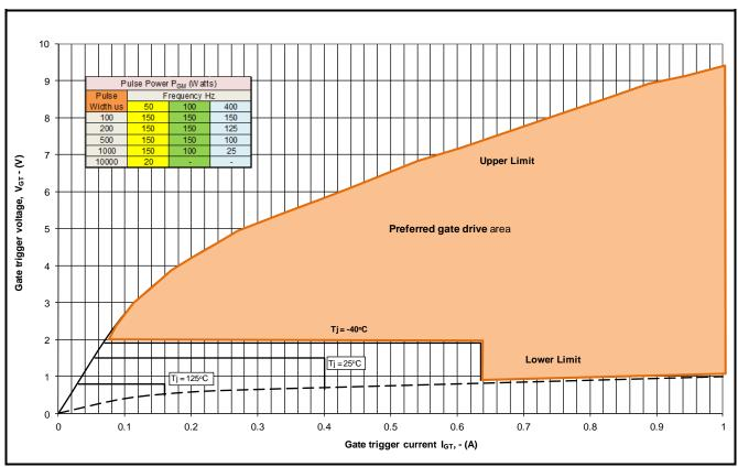
Fig14 Gate Characteristics
