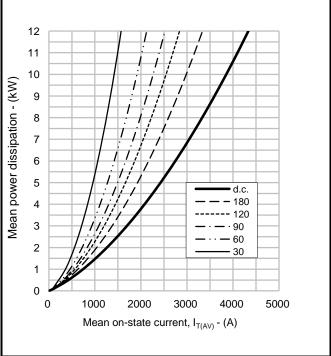
Fig.6 On-state power dissipation - rectangular wave
