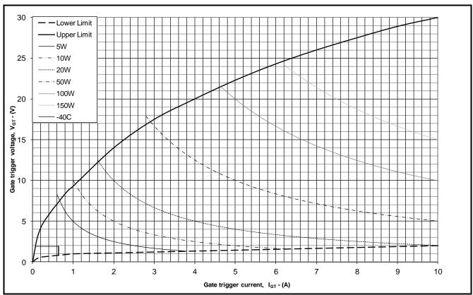
Fig. 15 Gate characteristics
