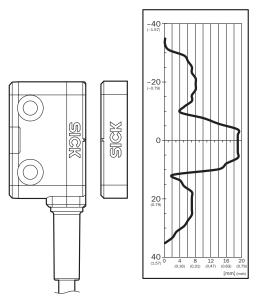
Safe switch on distance  $S_{Ao}$  14 mm.Pay attention to boundary areas in case of parallel approach: If the actuator moves laterally in relation to the surface of the sensor, a minimum distance of 10 mm must be maintained. This distance will prevent premature triggering due to the side approach areas.
