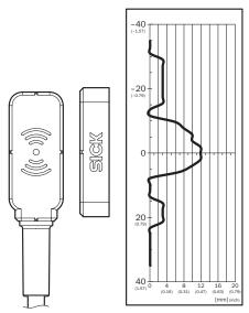
Safe switch on distance  $S_{Ao}$  9 mm.Pay attention to boundary areas in case of parallel approach: If the actuator moves laterally in relation to the surface of the sensor, a minimum distance of 4 mm must be maintained. This distance will prevent premature triggering due to the side approach areas.
