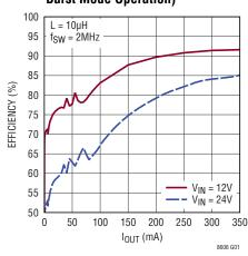
Efficiency (5V Output, Burst Mode Operation)
