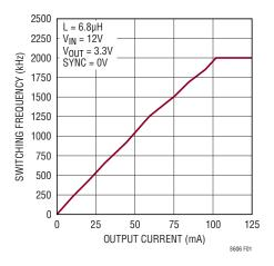
Figure 1. SW Burst Mode Frequency vs Output Current
