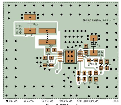
Figure 5. PCB Layout
