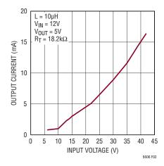
Figure 2. Full Switching Frequency Minimum Load vs V<sub>IN</sub> in Pulse Skipping Mode (MSOP ONLY)
