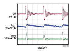
Figure 3. Burst Mode Operation
