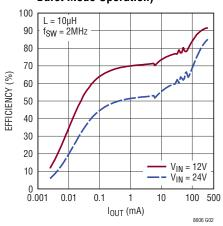
Efficiency (3.3V Output, Burst Mode Operation)
