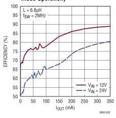
Efficiency (3.3V Output, Burst Mode Operation)
