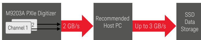
Figure 6. Streaming options (-CB0, -CB2) are proposed with a recommended host PC and SSD. Performance is guaranteed with specific configurations 3 .
