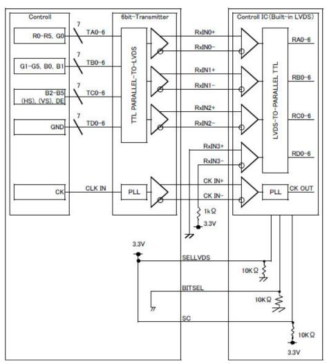
$\mbox{\ensuremath{\,\raisebox{-.3ex}{$\times$}}} SELLVDS$  signal line has 10 k  $\Omega$   $\,$  pulldown resister.
