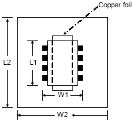
The PCB area  $L2 \times W2$  is 4 times of the IC's area  $L1 \times W1$ .
