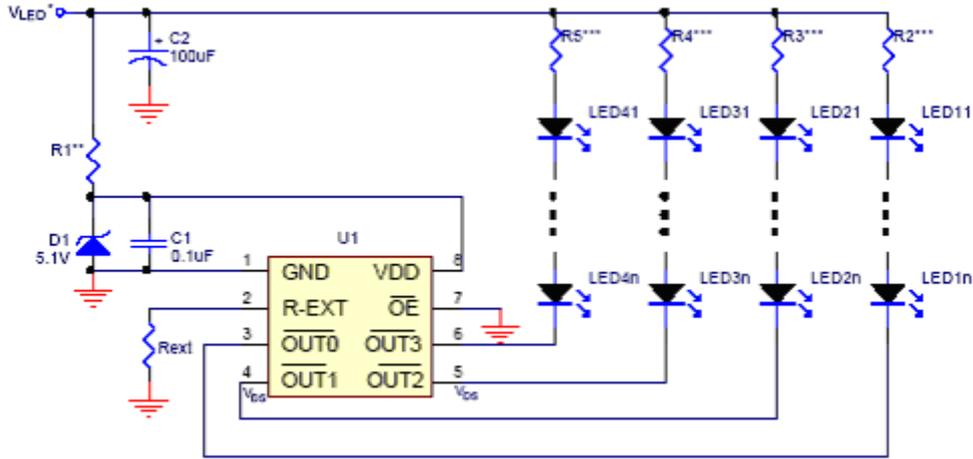
\*  $V_{LED} > V_{DS} + V_{F,LED} \times n$ ;  $V_{F,LED}$ : Forward voltage of LED; n: LED count
