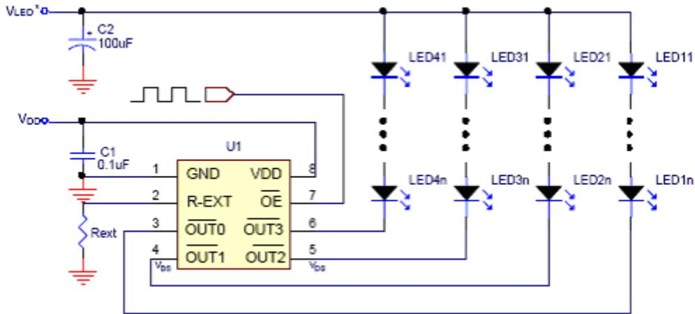
\*  $V_{LED} = V_{DS} + V_{F,LED} \times n$ ;  $V_{F,LED}$ : Forward voltage of LED; n: LED count
