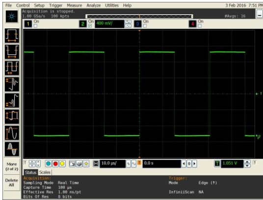
Figure 3. LVC MOS Output Swing ( V_{DD} = 1.8\text{V} )
