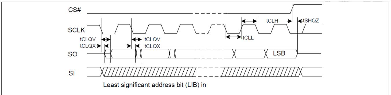
Figure15. Output Timing
