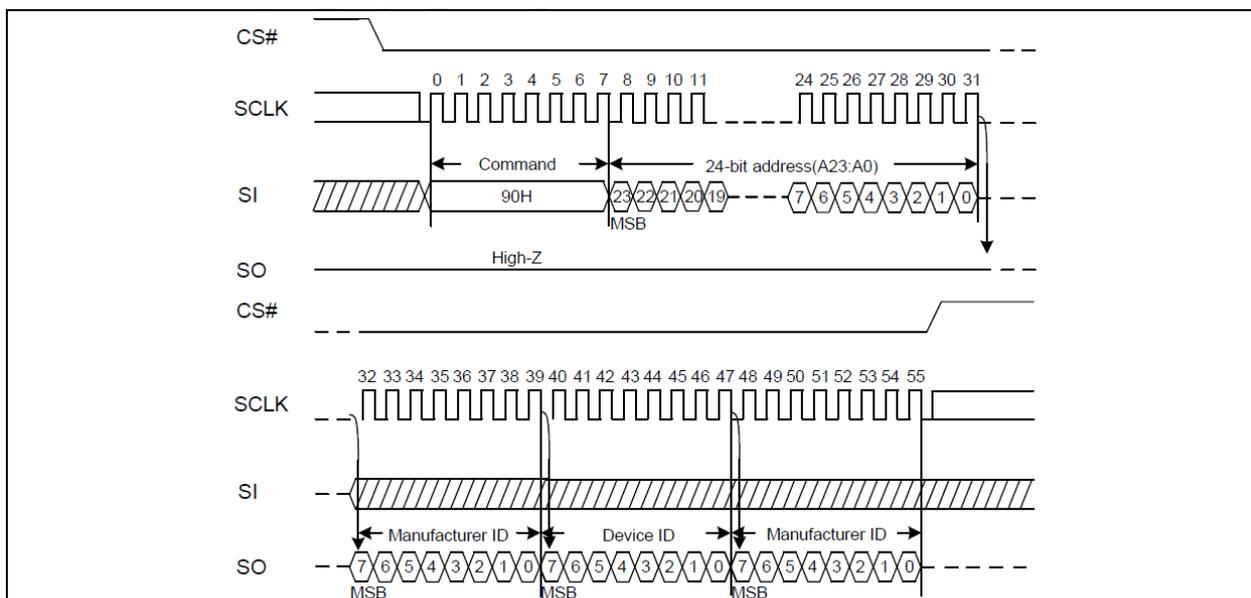
Figure11. Read Manufacture ID/ Device ID Sequence Diagram
