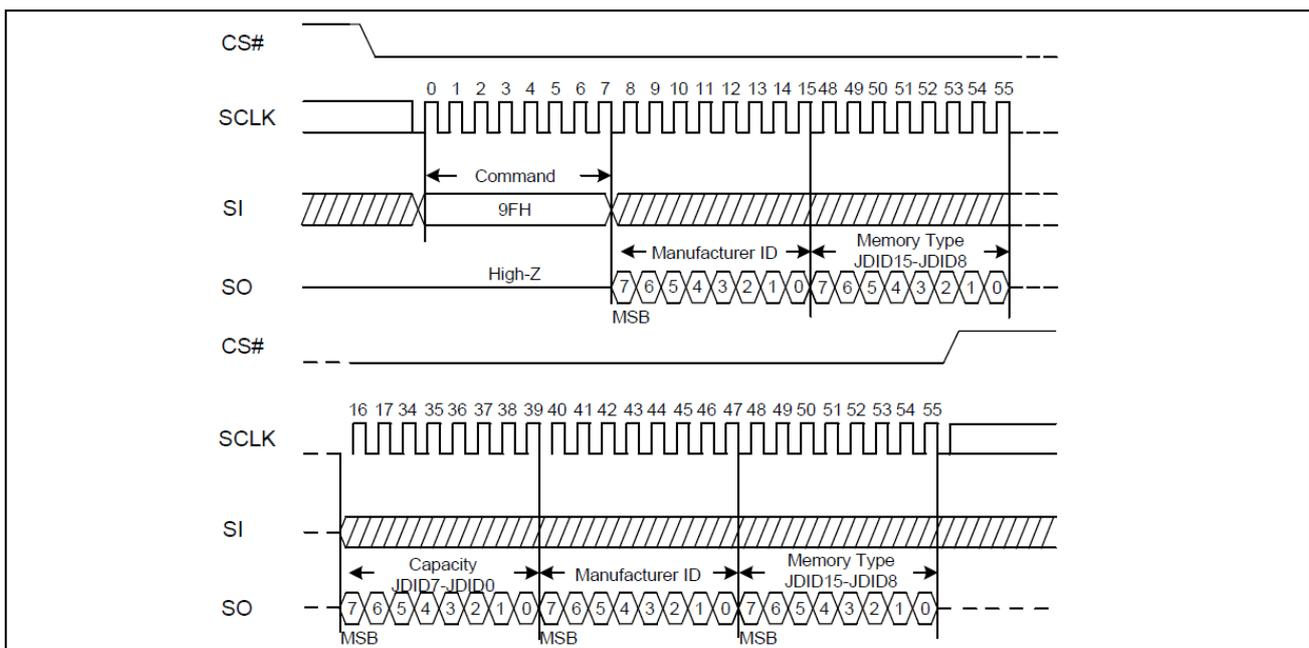
Figure12. Read Identification ID Sequence Diagram
