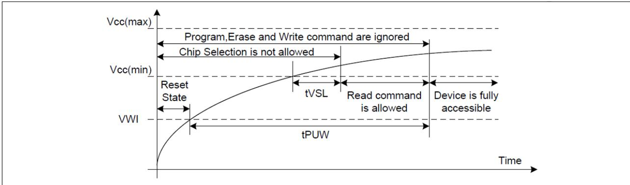
Table3. Power-Up Timing and Write Inhibit Threshold
