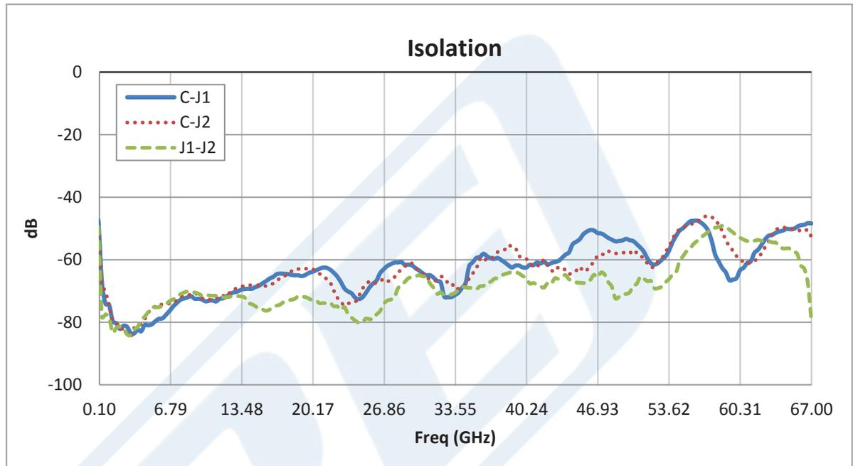
Absorptive SPDT PIN Diode Switch Operating From 100 MHz to 67 GHz Up to +27 dBm and 1.85mm from Pasternack Enterprises has same day shipment for domestic and International orders. Our RF, microwave and millimeter wave products maintain a 99% availability and are part of the broadest selection in the industry.
