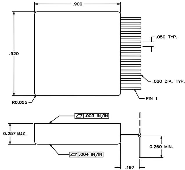
**Figure 8 – Space Saving Surface Mount Lead Bend.**
