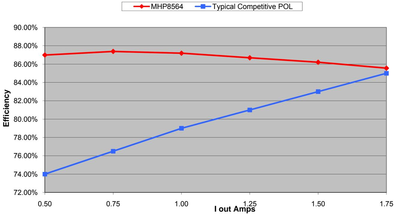
**Figure 12 – MHP8564 Typical Efficiency Curves (Vin = 5V)**
