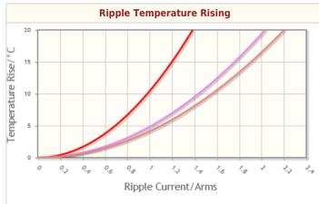
C2012X7R1H105K125AB(100kHz) C2012X7R1H105K125AB(500kHz) C2012X7R1H105K125AB(1MHz)
