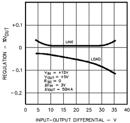
Figure 4. Regulations vs. Input-Output Voltage Regulation
