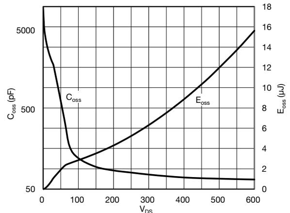
**Fig. 6 - C<sub>oss</sub> and E<sub>oss</sub> vs. V<sub>DS</sub>**
