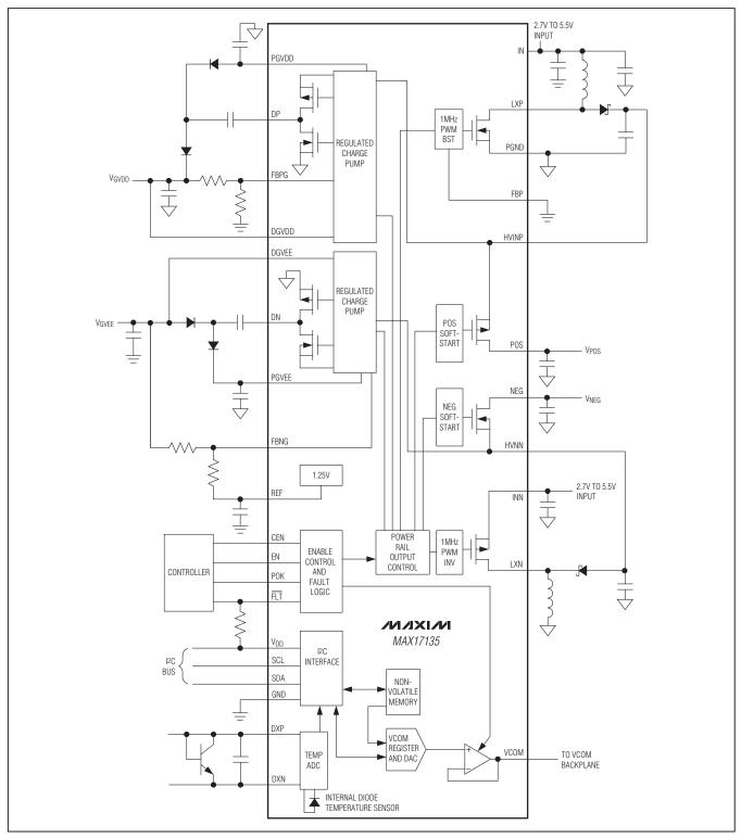
Figure 3. Functional Diagram
