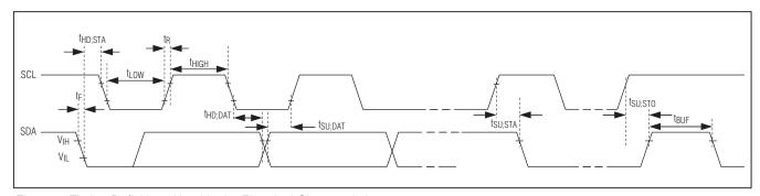
Figure 1. Timing Definitions Used in the Electrical Characteristics
