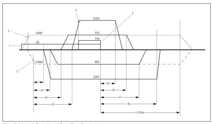
Figure 5. Adjustable Power-Up and Power-Down Sequencing
