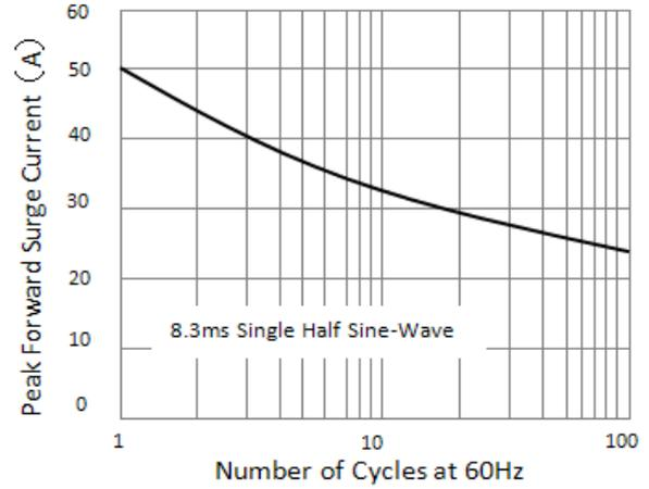
Figure 2. Maximum Non-Repetitive Peak Forward Surge Current
