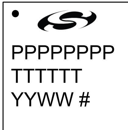
Figure 6.3. QFN28 Package Marking
