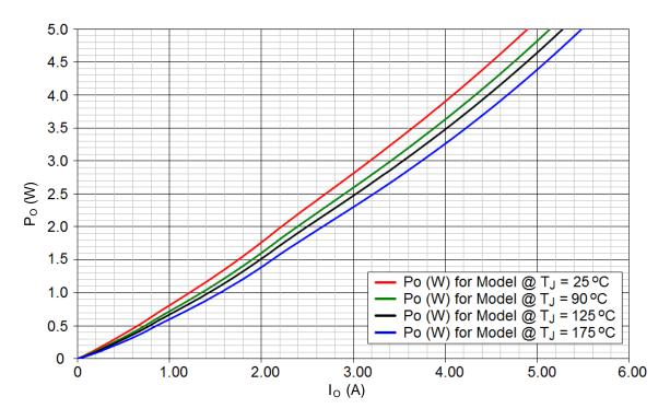
FIGURE 2 Rectifier Power vs Io (Average Forward Current)
