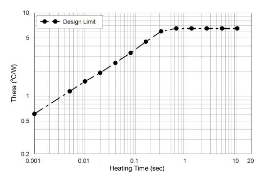
FIGURE 1 Maximum Thermal Impedance
