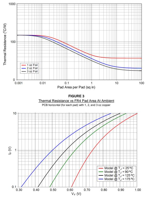
FIGURE 4 Forward Voltage vs Forward Current
