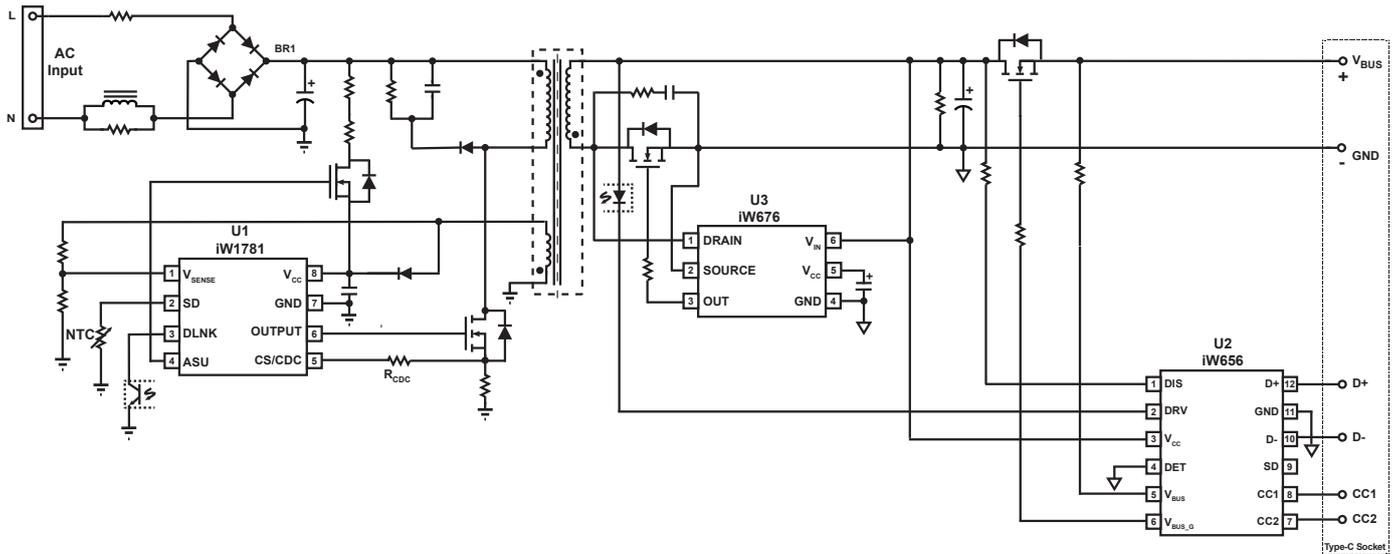
**Figure 2.1 : iW1781 typical application circuit for standard USB PD with optional QC2.0/QC3.0 enabled (Using iW656 as Secondary-Side Controller for USB PD and iW676 as Synchronous Rectifier Controller.)**
