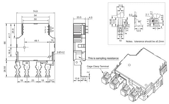
Remark: In case of no tolerance shown in outline dimension: outline dimension  $\leq$ 1mm, tolerance should be  $\pm$ 0.2mm; outline dimension >1mm and  $\leq$ 5mm, tolerance should be  $\pm$ 0.3mm; outline dimension >5mm, tolerance should be  $\pm$ 0.4mm.
