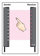
The "red" Job LEDs light in case of picking errors. The function LED "Func" will also turn "red" to indicate a picking error.
