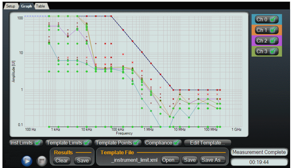
Figure 16. Jitter tolerance graph view.
