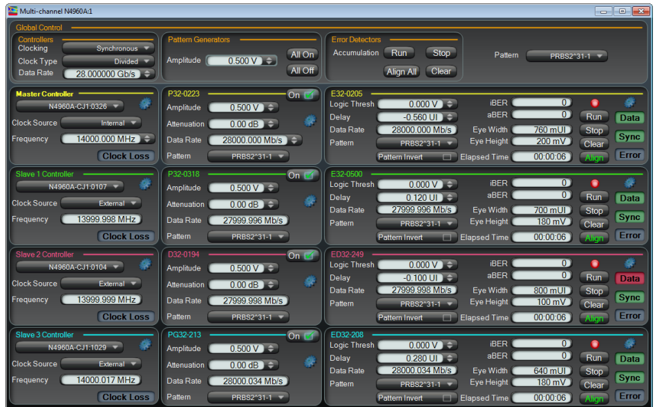
Figure 10. N4980A multi-channel BER measurement interface.
