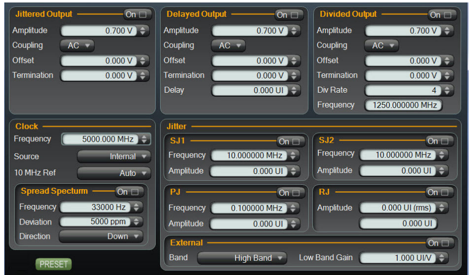
Figure 9. N4980A multi-instrument BERT software.
