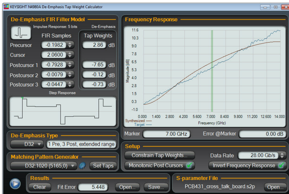
Figure 7. De-emphasis tap weight calculator.
