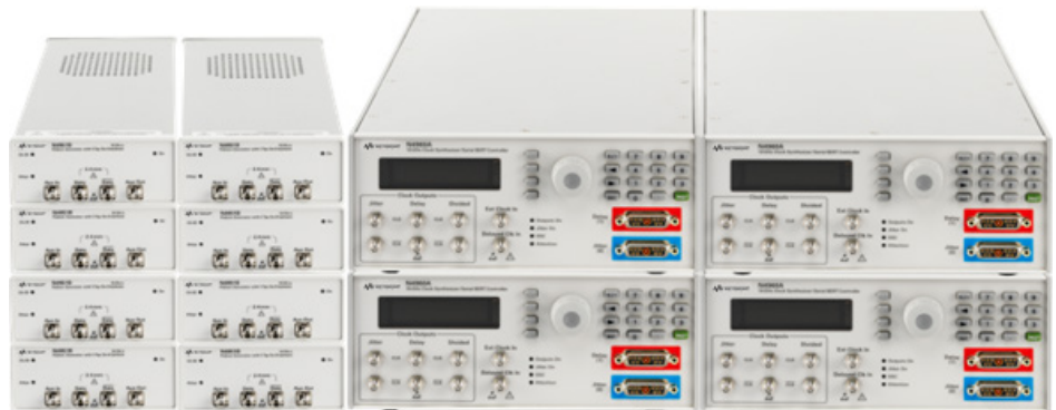
Figure 11. N4960A multi-channel hardware configuration.
