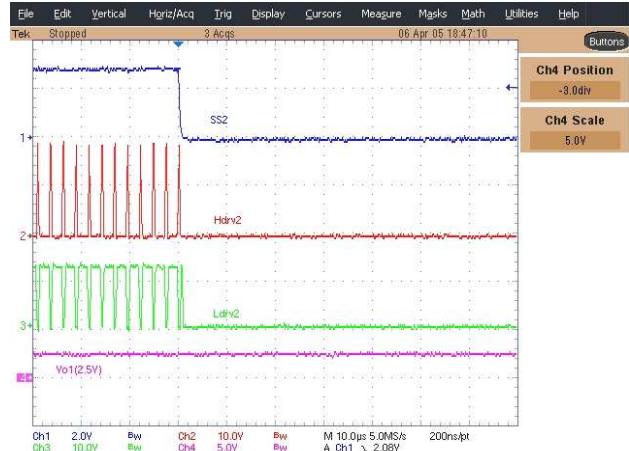
Figure 18 - SS2 pin shorted to Gnd Ch1: SS2, Ch2: Hdrv2, Ch3: Ldrv2, Ch4: Vo1
