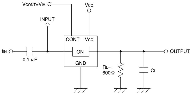
\* Input by sine wave ( $V_{IN}=0\text{dBm}$ ,  $f=1\text{MHz}$ )
