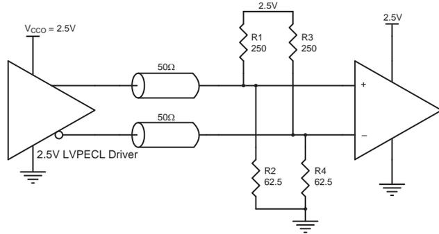
Figure 26: 2.5V LVPECL Driver Termination Example
