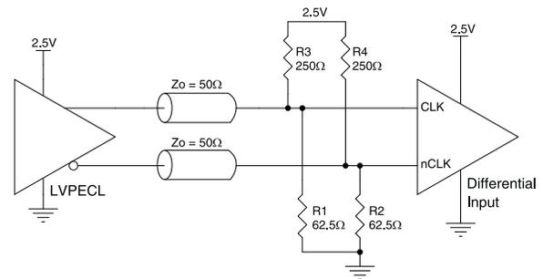
Figure 20: CLK/ nCLK Input Driven by a 2.5V LVDS Driver
