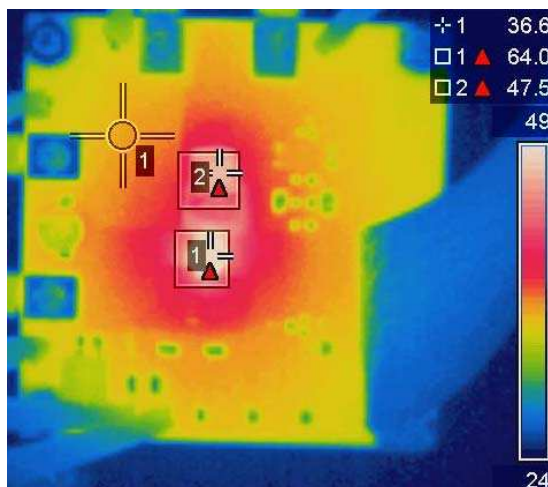
Figure 21: Thermal Image at VIN = 12V, IOUT = 6A (IR3473: 64°C, Inductor: 48°C, PCB: 37°C)
