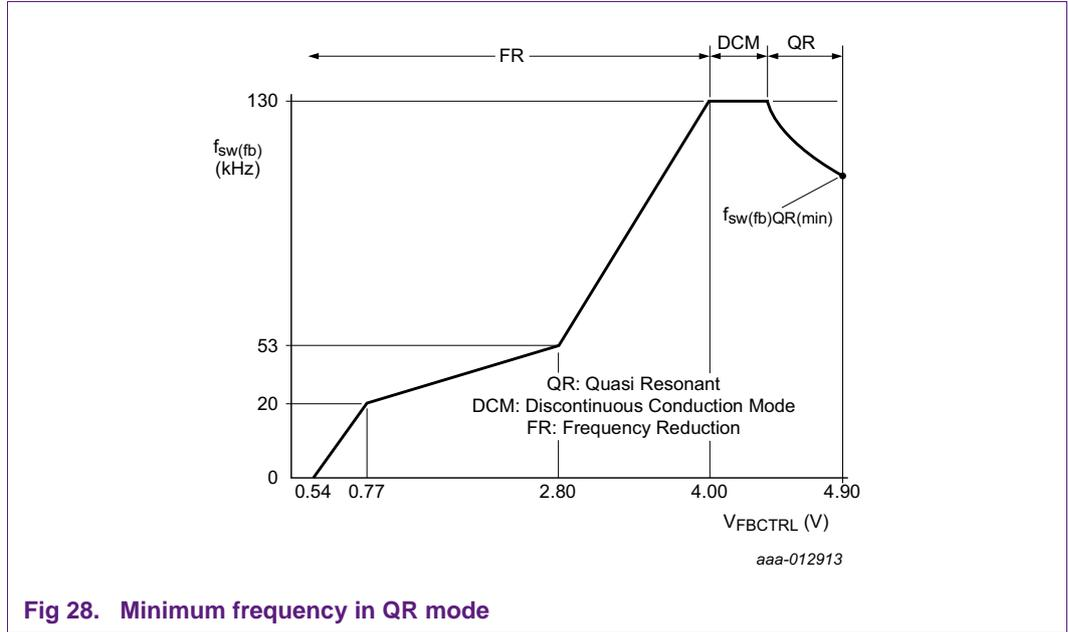
Fig 28. Minimum frequency in QR mode
