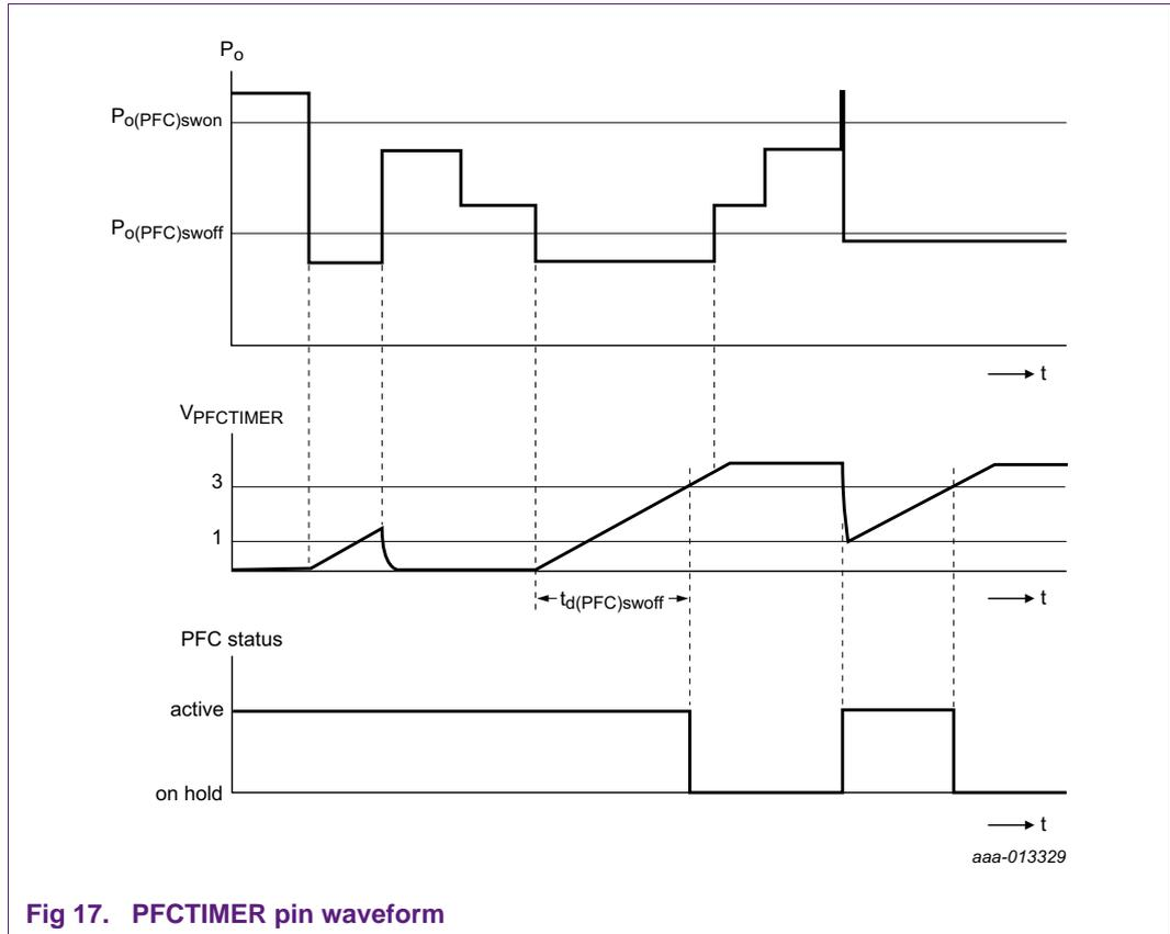
Fig 17. PFCTIMER pin waveform
