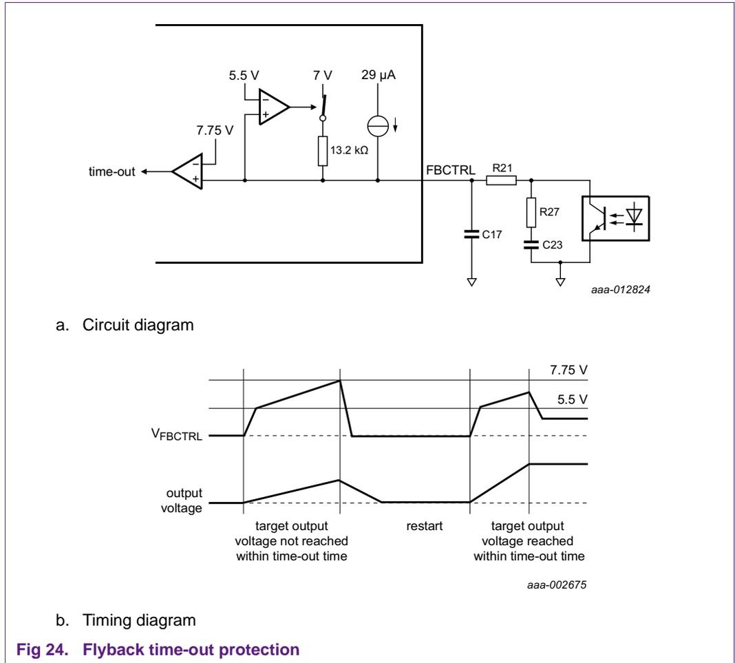
A noise filter (C17 = 220 pF; R21 = 10 Ω) located close to pin FBCTRL avoids interference by PFC MOSFET switching or HF noise (e.g. GSM phone). Resistor R27 and capacitor C23 set the time delay for V<sub>FBCTRL</sub> to reach 7.75 V. Resistor R27 is required to separate the relatively high-value time-out capacitor C23 from the control loop response. The value of resistor R27 must be > 30 kΩ.
