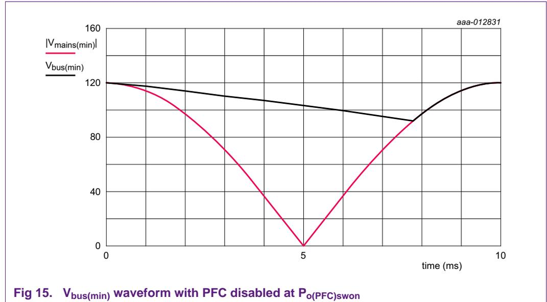
Fig 15.  $V_{bus(min)}$  waveform with PFC disabled at  $P_{o(PFC)swon}$
