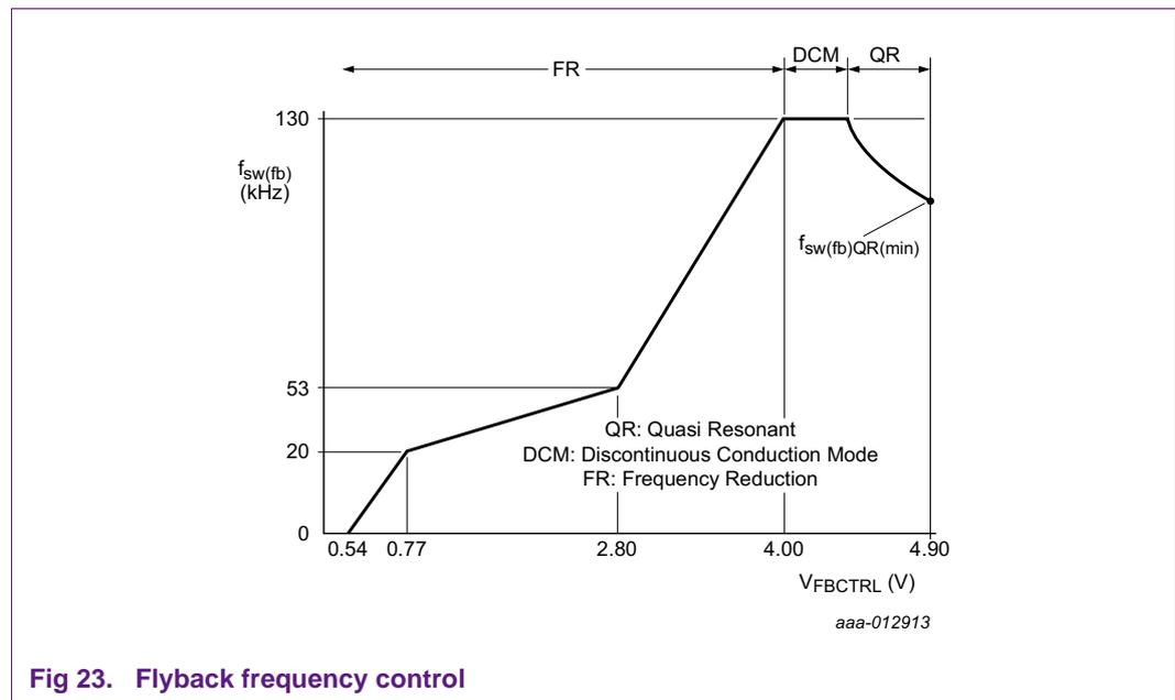
**Fig 23. Flyback frequency control**
