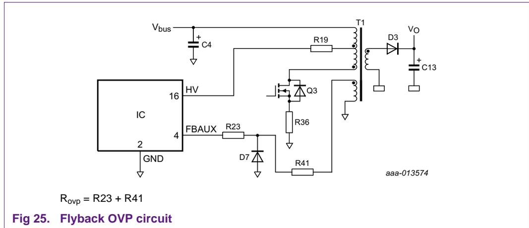
An internal integrator filters noise and spikes. The output of the integrator connects to a counter. The counter prevents false OVP detection which can occur during ESD or lightning events.
