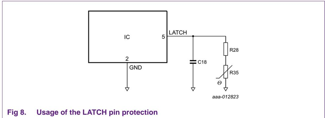
**Fig 8. Usage of the LATCH pin protection**
