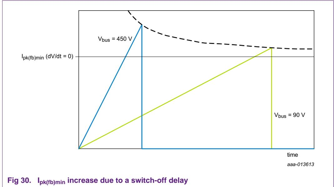
$\Delta I_{pk(fb)}$  results in a voltage on resistor R36 which must be compensated as a function of  $V_{bus}$  by  $I_{R20}$  through resistor R31:
