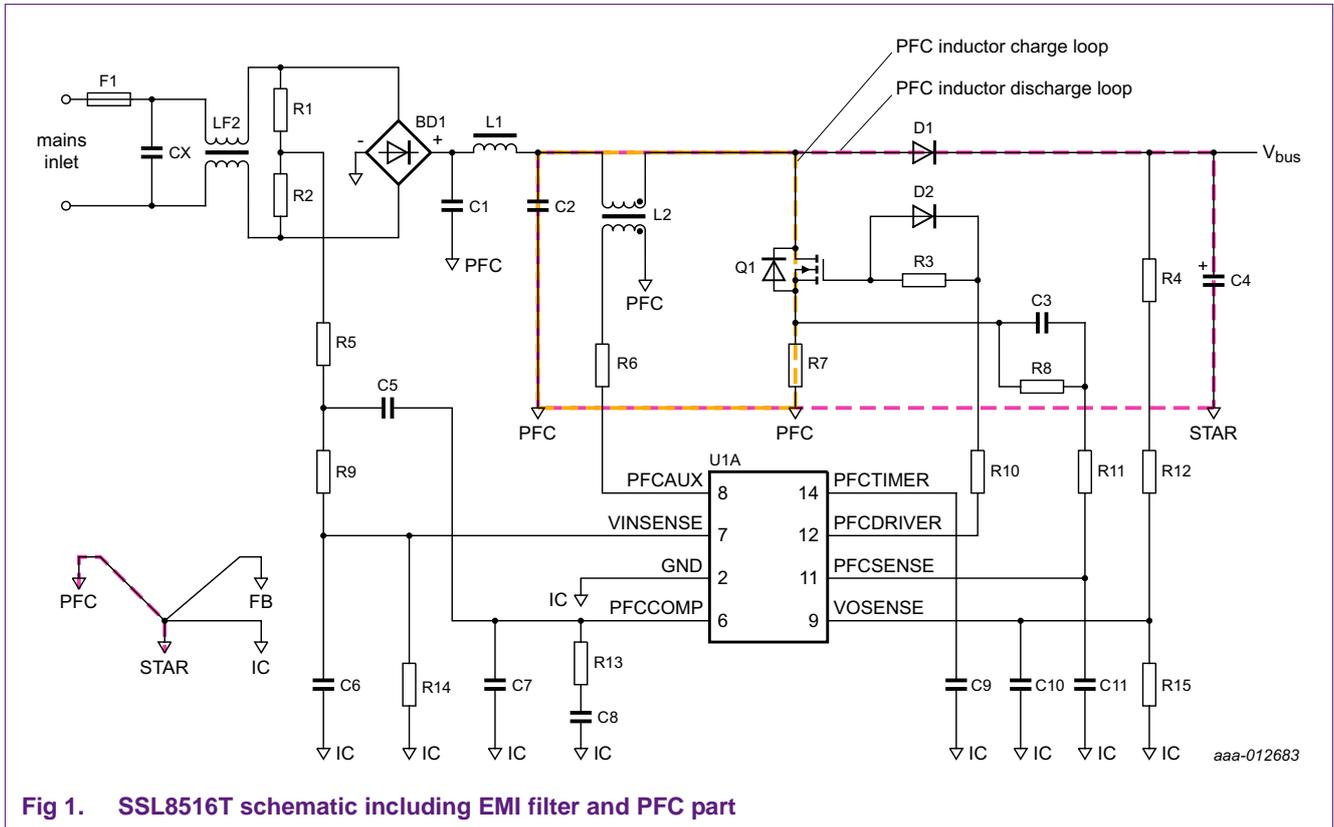
Fig 1. SSL8516T schematic including EMI filter and PFC part
