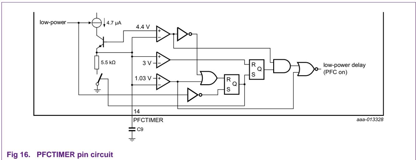
Fig 16. PFCTIMER pin circuit
