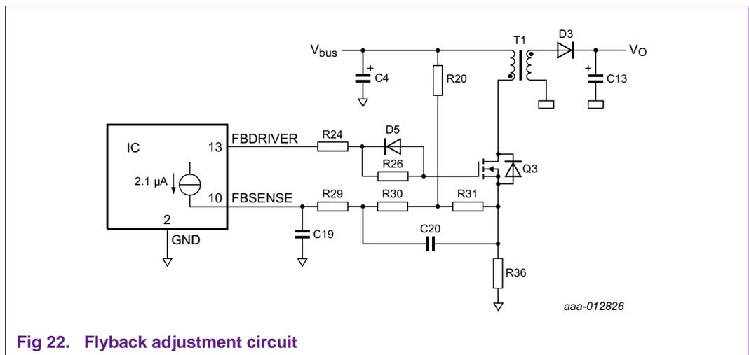
Fig 22. Flyback adjustment circuit
