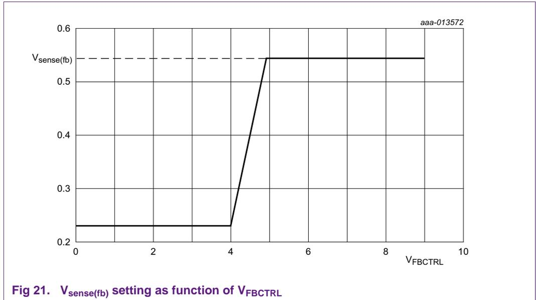
Fig 21.  $V_{sense(fb)}$  setting as function of  $V_{FBCTRL}$
