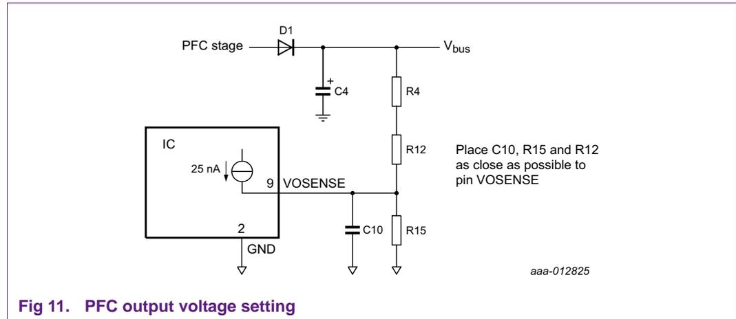
Fig 11. PFC output voltage setting
