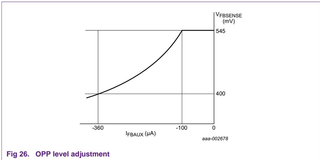
**Fig 26. OPP level adjustment**
