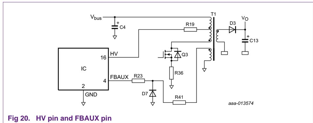
Fig 20. HV pin and FBAUX pin
