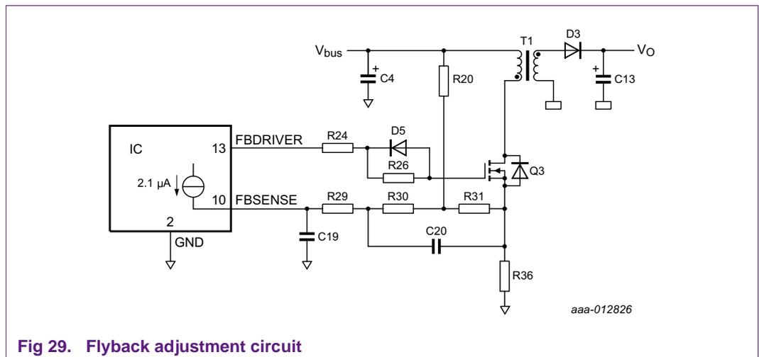
Fig 29. Flyback adjustment circuit
