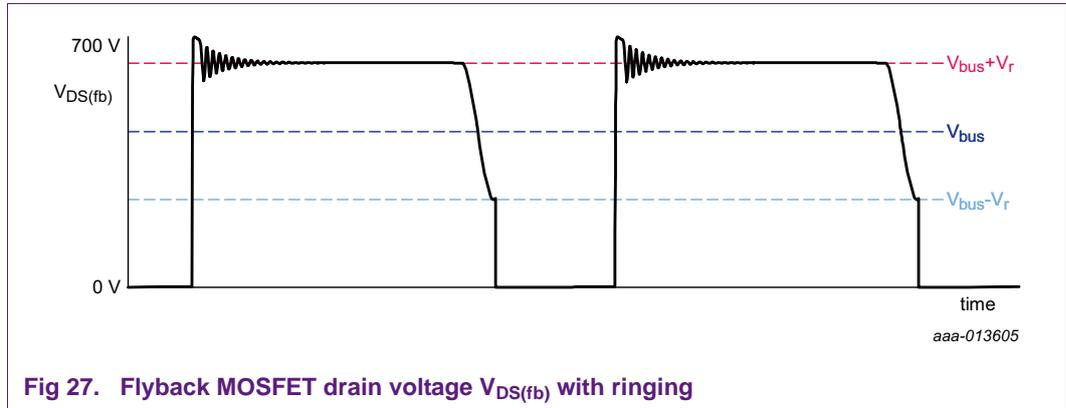
Fig 27. Flyback MOSFET drain voltage  $V_{DS(fb)}$  with ringing
