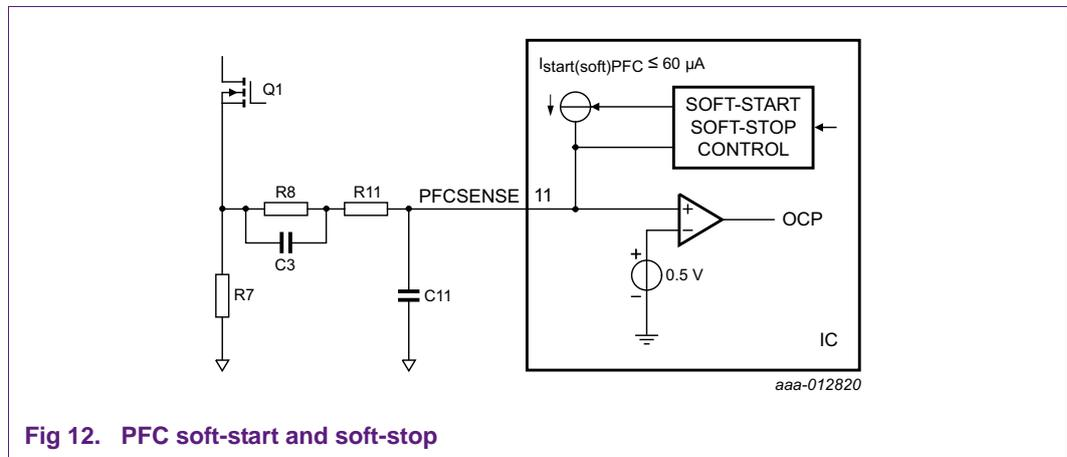
Fig 12. PFC soft-start and soft-stop
