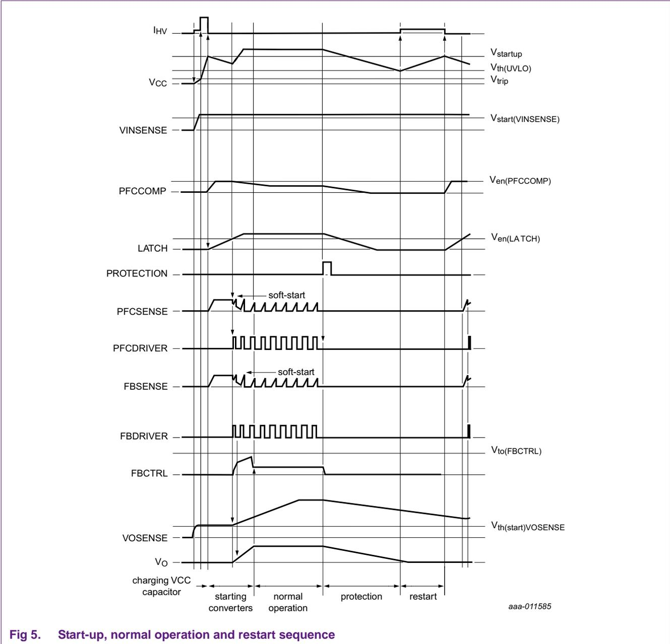
Fig 5. Start-up, normal operation and restart sequence
