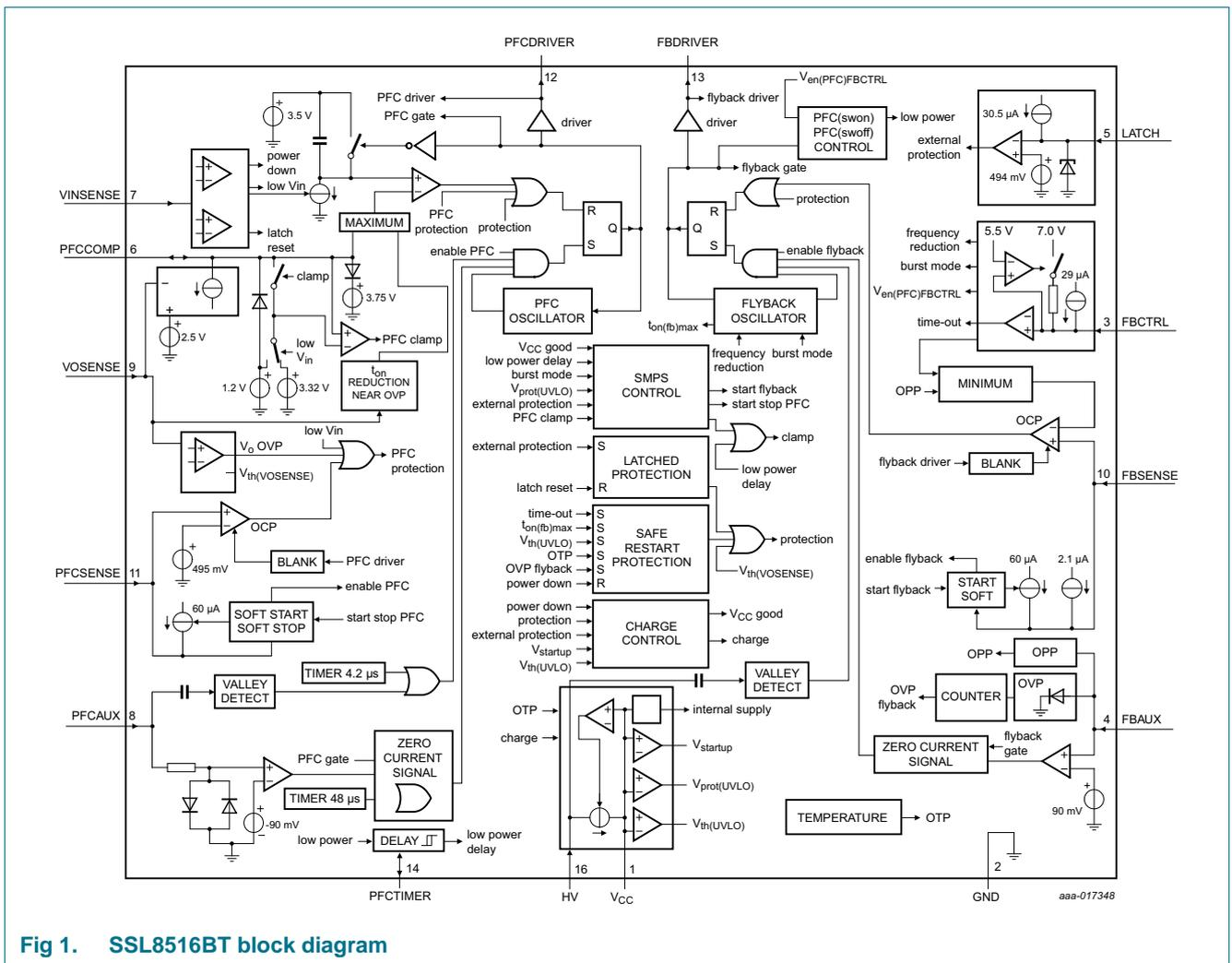
Fig 1. SSL8516BT block diagram
