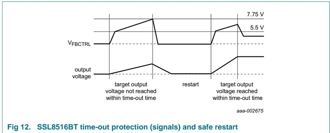
Fig 12. SSL8516BT time-out protection (signals) and safe restart
