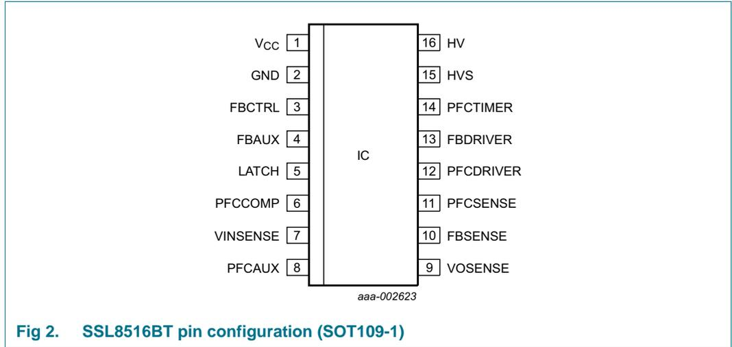
Fig 2. SSL8516BT pin configuration (SOT109-1)
