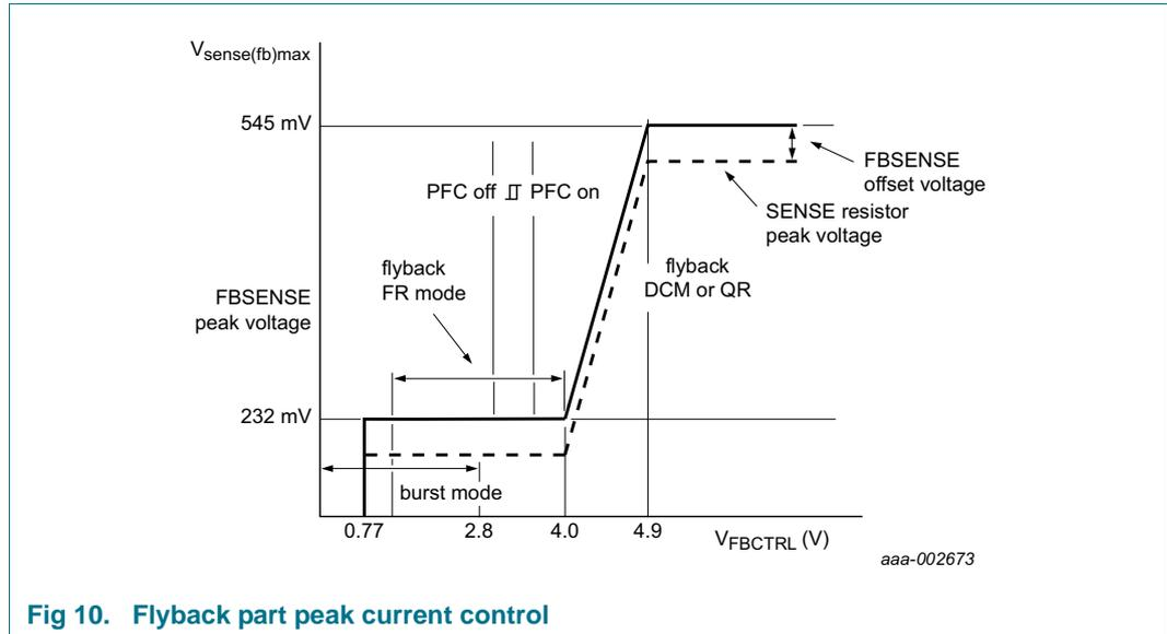
Fig 10. Flyback part peak current control
