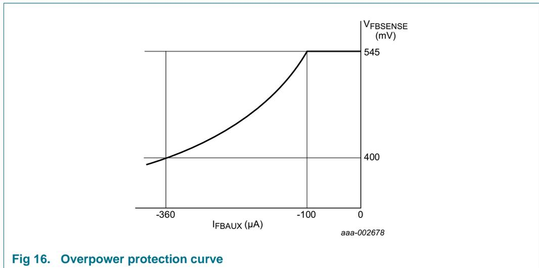
Fig 16. Overpower protection curve
