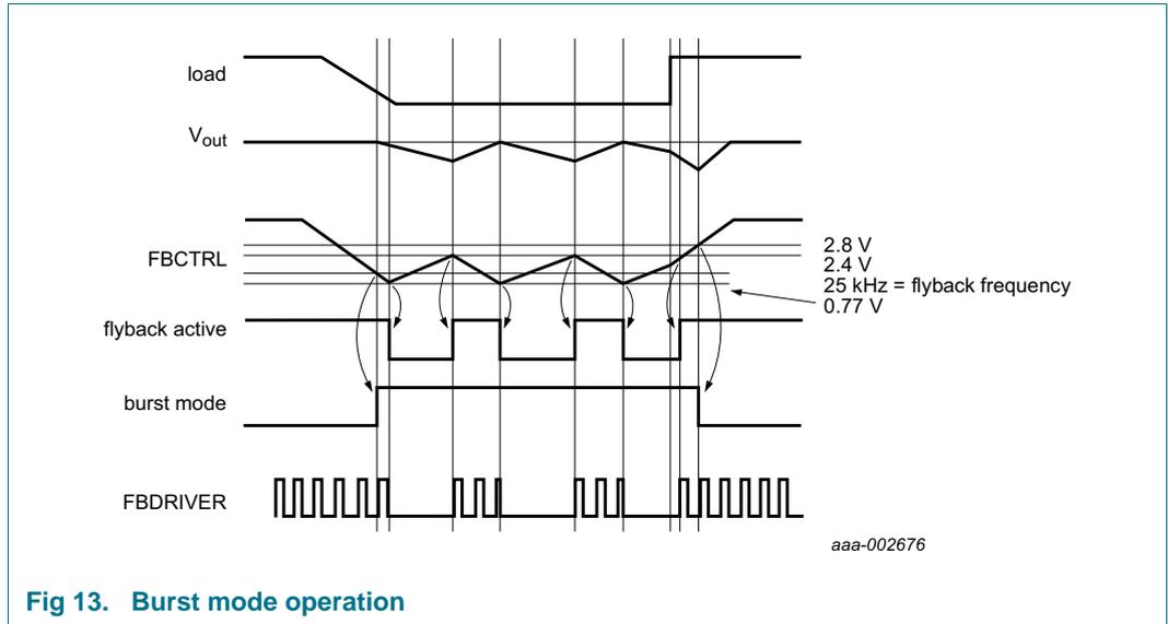
Fig 13. Burst mode operation
