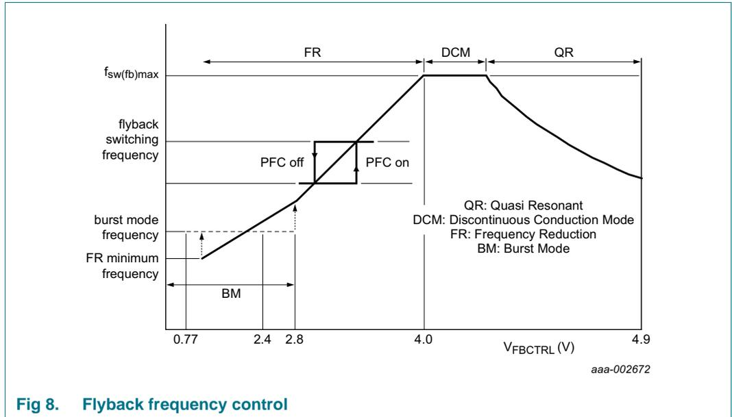
Fig 8. Flyback frequency control
