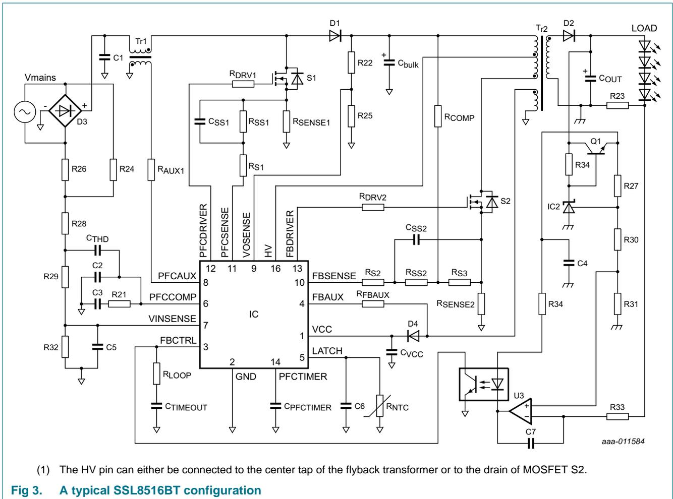
Fig 3. A typical SSL8516BT configuration
