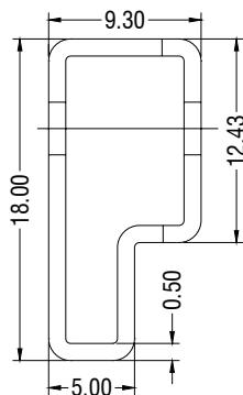
Tube length (14 Pin DIP) : 520mm $\pm$ 2mm.
